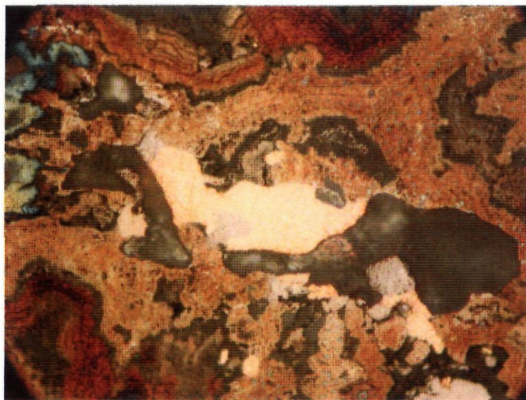
Figure 15 F866A, REF. Same area as above figure . Yellow electrum intergrown with pale grey tellurbismuthite , surrounded by tarnished marcasite after pyrrhotite.
