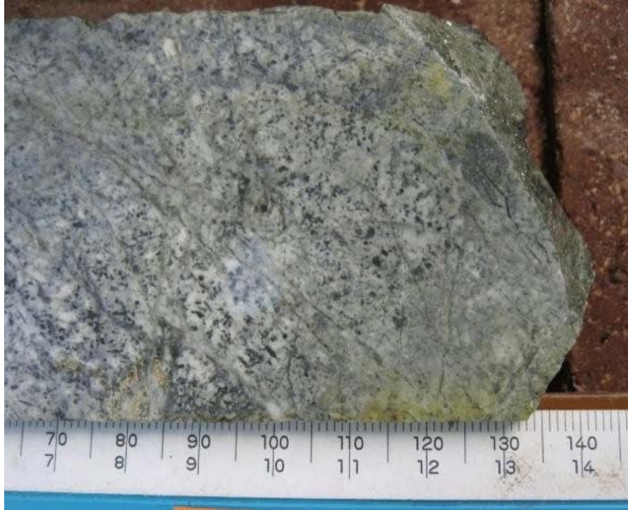
Figure 13. Mineralized hornblende crowded feldspar diorite, brecciated zone next to phonolite dyke in GK07-04. Disseminated pyrite and pyrrhotite present in rock and in frequent microveins. The pyrite on the exposed fracture surface is in cubic crystal form.
