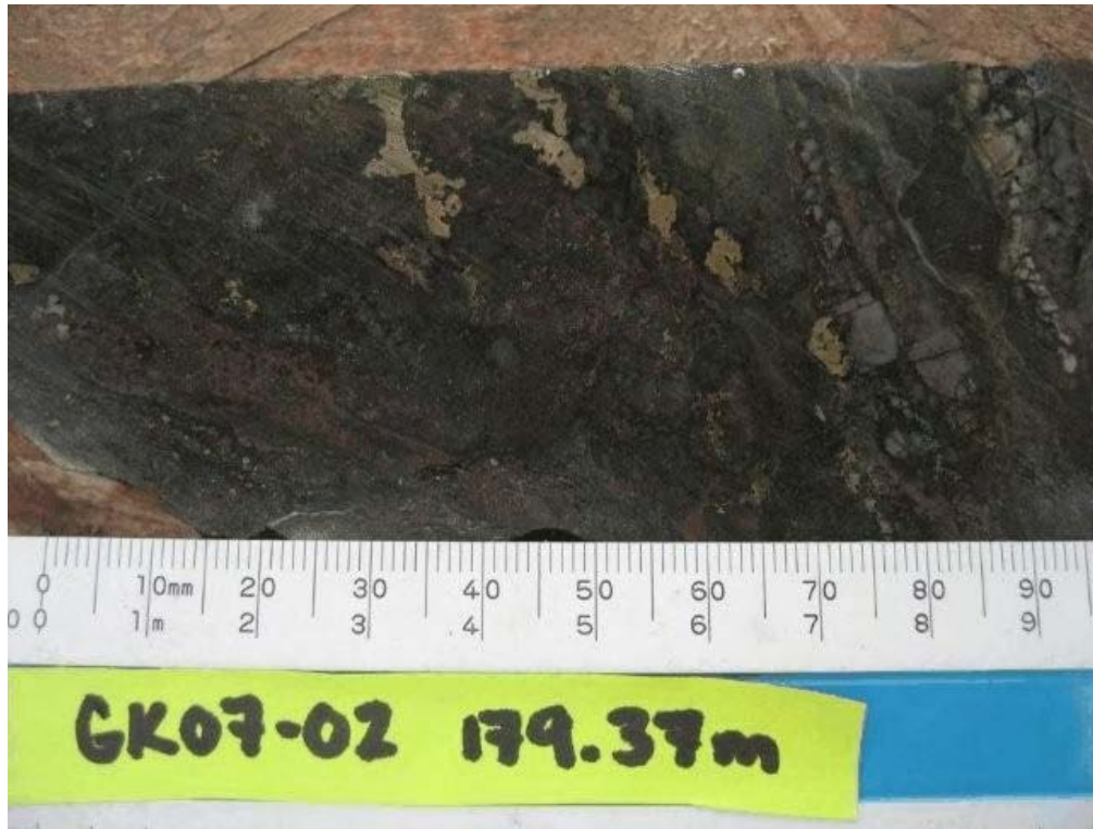
Figure 19. Brecciated feldspathic fine tuff, matrix is fine grained chlorite, quartz with disseminated to semi-massive pyrite and sphalerite and local pyrrhotite, containing 1.165 g/tonne Au, 32.9 g/tonne Ag, 3220 ppm Pb and 15300 ppm Zn over 0.20 metres from 179.37 to 179.57metres; GK07-02.
