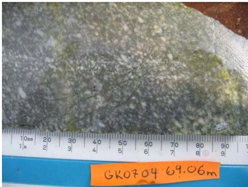
Figure 12. Stained hornblende crowded feldspar diotite, plagioclase feldspar in a matrix of subordinate and finer grained hornblende, potassium feldspar and quartz, shows typical lack of potassium feldspar in the GK diorites; GK07-04.
