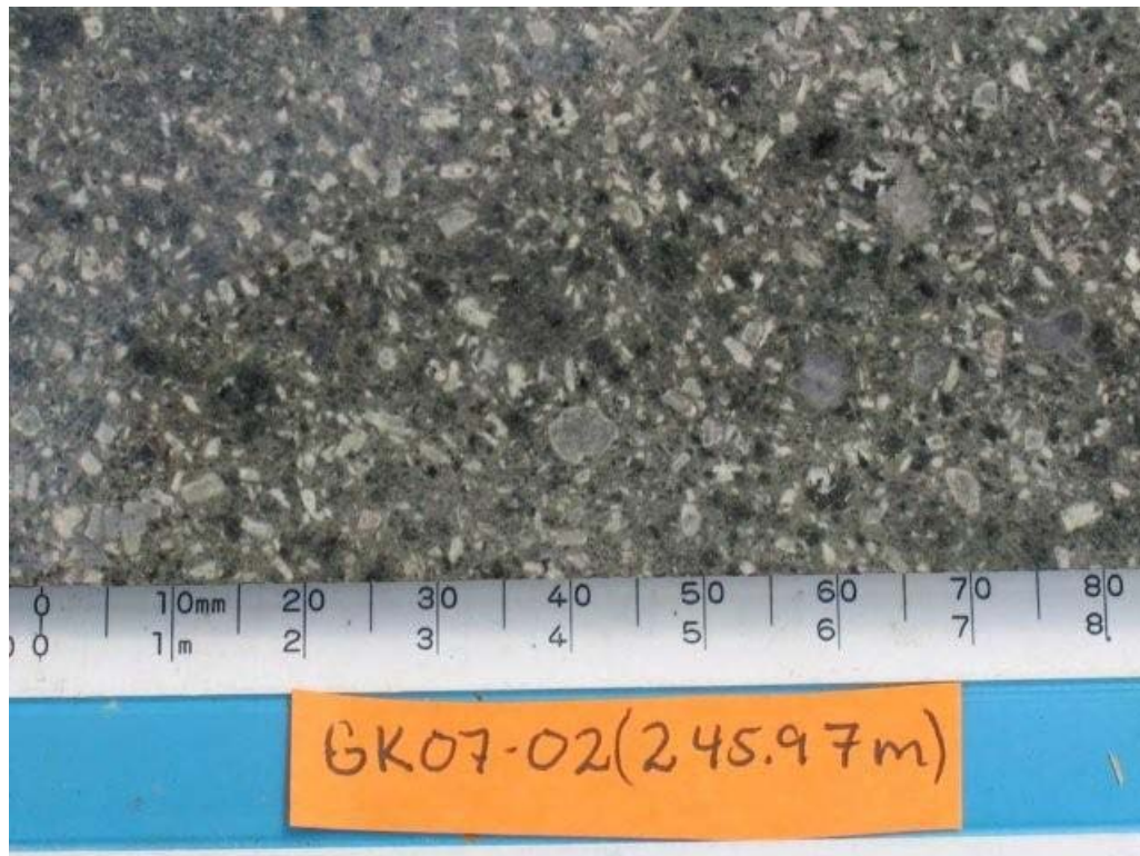
Figure 14. Typical porphyritic phonolite/latite dyke, blocky to tabular habit of white weathering plagioclase feldspar phenocrysts and amorphous habit of black pyroxene phenocrysts; GK07-02.
