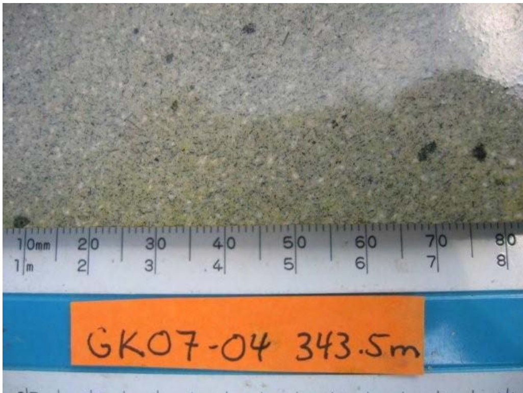
Figure 15. Stained dyke section, very fine grained, beige, acicular hornblende and hollow needle texture. Plagioclase feldspars prominent, staining shows lack of potassium feldspars (hornblende needle feldspar porphyry dyke); GK07-04.
