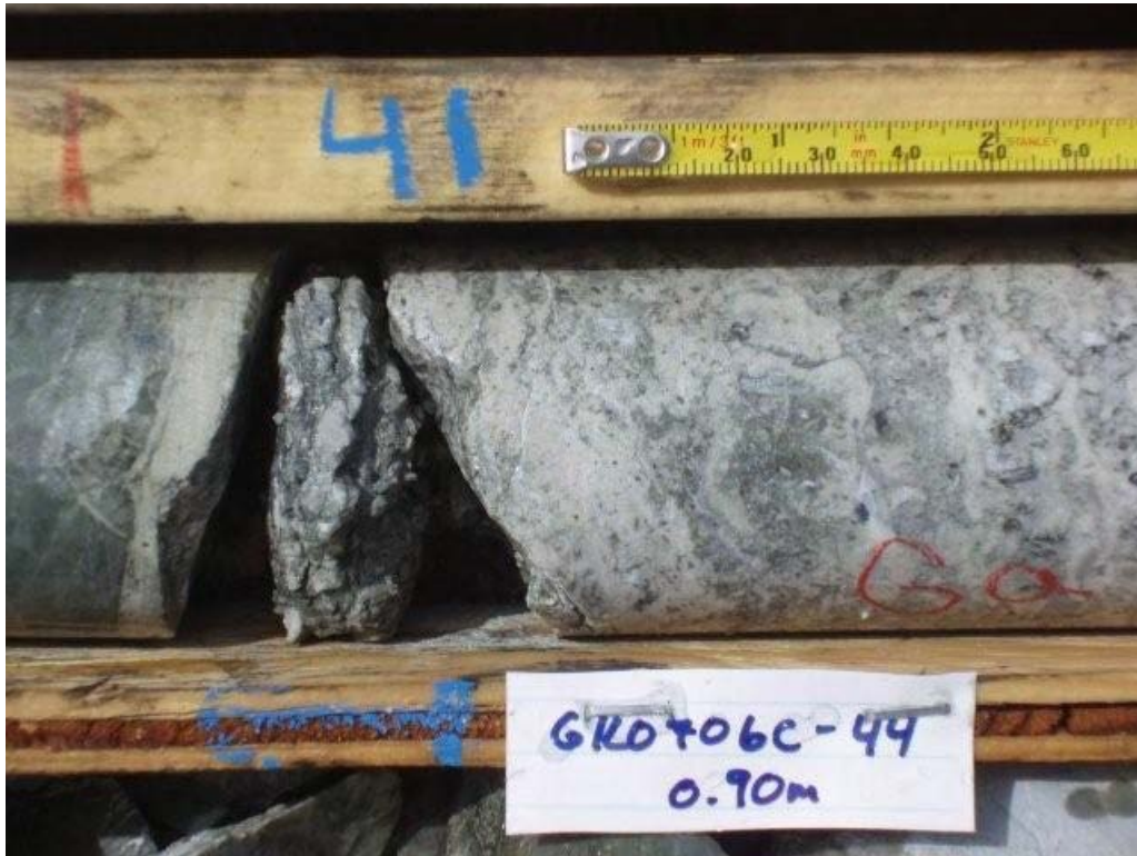
Figure 23. Bleached (albitized?) and brecciated feldspathic fine tuff, mineralization includes disseminated pyrite and 1 mm blebs of galena, adjacent to a 2.0 cm (minimum) gouge zone which is preceded by locally brecciated tuff; GK0706
