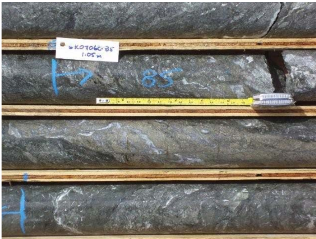
Figure 24. Brecciated feldspathic fine tuff mineralized by disseminated pyrite (up to 25%) and cut by late white calcite veinlets. Sample 85 assayed 0.379 g/tonne Au , 3.8 g/tonne Ag and 1110 ppm As, between 193.10 and 194.15 metres, followed by #86 containing 2.45 g/tonne Au, 24 g/tonne Ag and > 10,000 ppm As between 194.15 and 194.80 metres; GK07-06.
