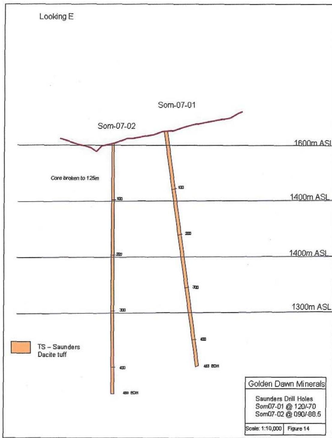
Som-07-01 is shown on Figure 13. The hole was collared on September 13, 2007, drilled to 453.15 m, and terminated on September 23, 2007. A section of DDH Som-07-01, together with Som-07-02, viewed to the east, is given in Figure 14.
