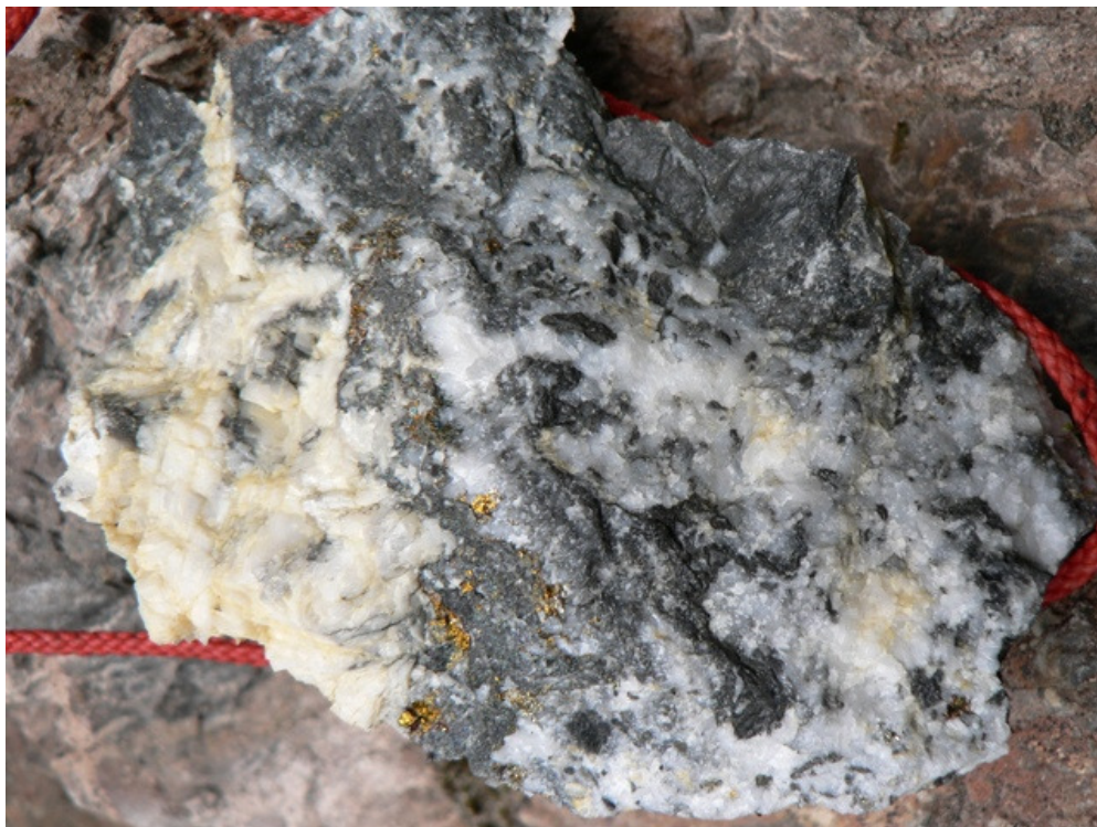
Picture 3 & 4. The silicified phyllite and quartz/carbonate veining that contains 1-5% sulfides at the entrance to the Wedge Project Adit.
