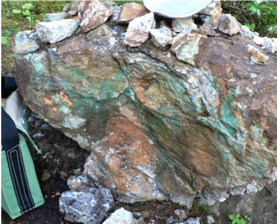
Picture 10. In general there is only very minor weathering of the Wedge structure however along some fractures copper oxide staining can be seen from the weathering sulfides. This is also associated with hematite staining nearer the massive quartz veining.
