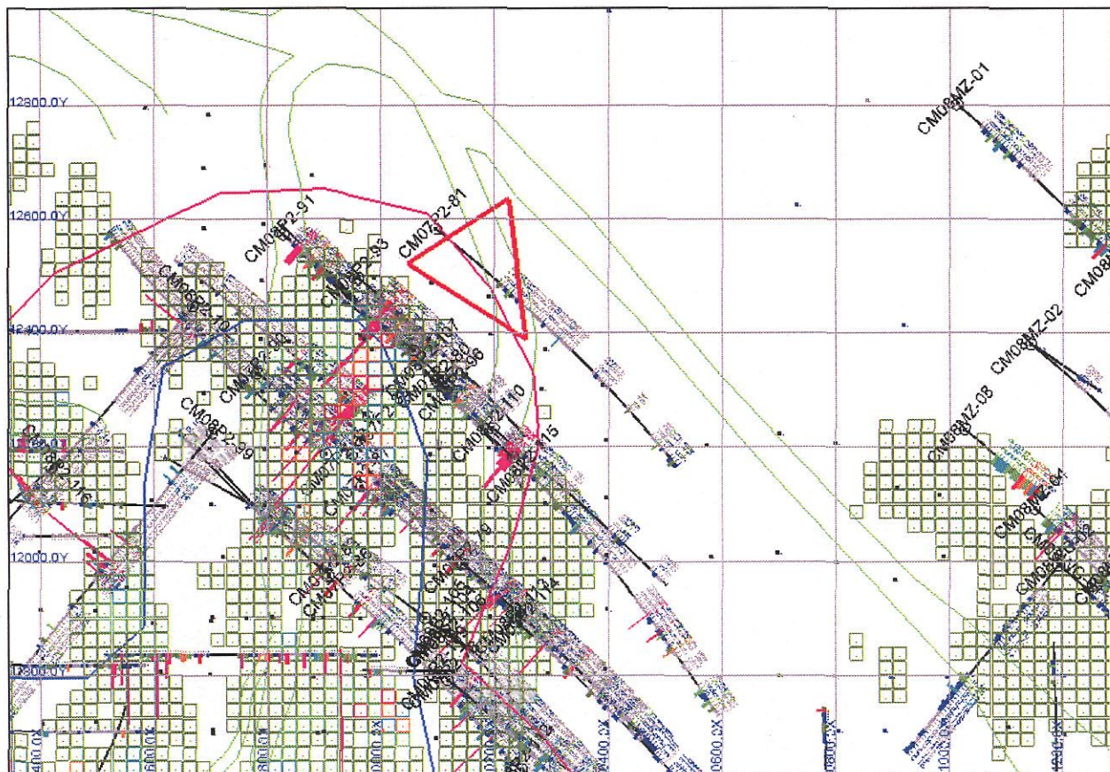
Figure 3.1 Plan map of the northeastern end of Pit 2, showing drill-holes, resource blocks (green), the edge of existing Pit 2 (blue), the edge of the current super-pit (magenta) and the outline of the Annie Fr (red)
