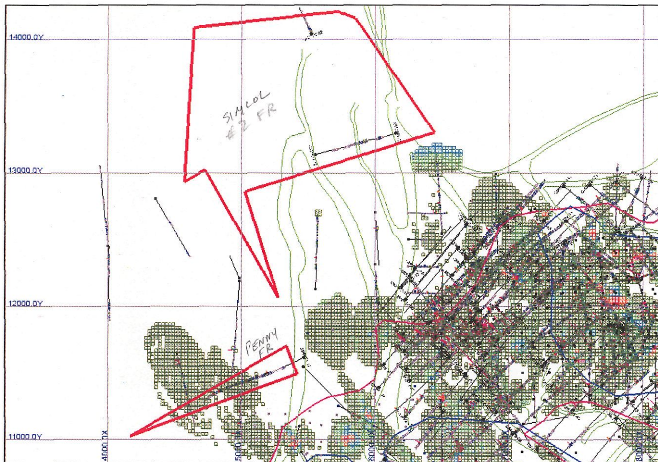
Figure 3.3 Plan map from the western end of Pit 2 showing drill-holes, resource blocks (green), the edge of existing Pit 2 and Pit 1 (blue), the edge of the current super-pit (magenta) and the outline of the Simcol #2 Fr and Penny Fr (red).
