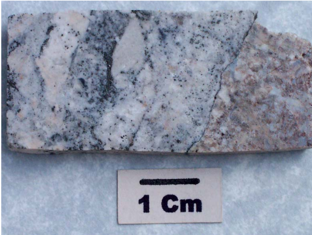
Sample 07-BON-ALT-02. Small slab of 'alteration/vein', probably a hydrothermal breccia (left 2/3) and altered wall rock volcanic (light pinkish brown, right 1/3). Material analyzed with XRD was mixture of grayish and pinkish material with disseminated pyrite from the vein-breccia (left).
