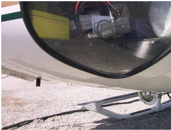
Figure 6. Digital video camera typical mounting location.
