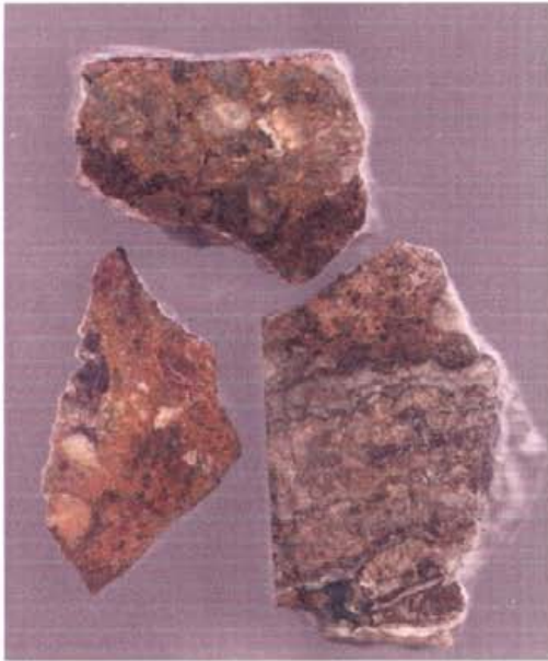
Plate 1: Schmitt Zone Breccia: Note discrete silicified fragments which are in part jasperoidal. These appear to be derived from previously formed epithermal veins and suggest that this zone represents a breccia pipe or diatreme.
