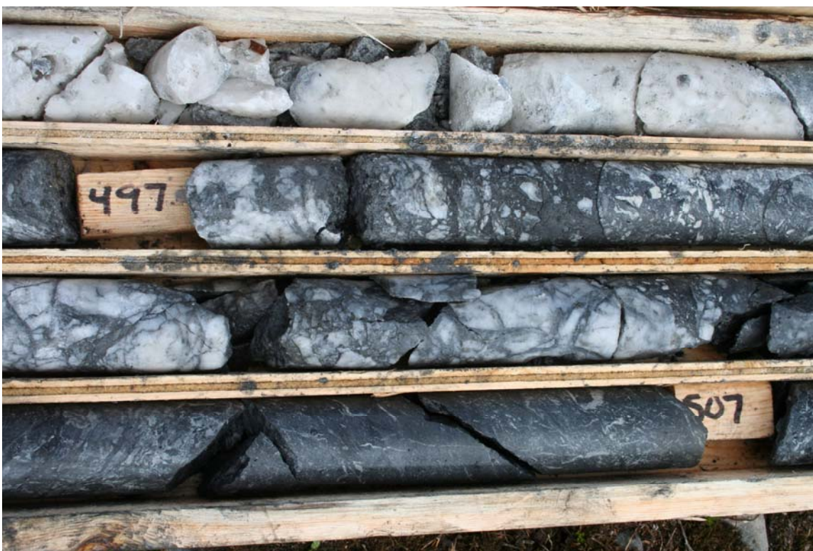
Figure 11 - 2006 Drill Core - Quartz cemented as a breccia from SDN-06-03.
