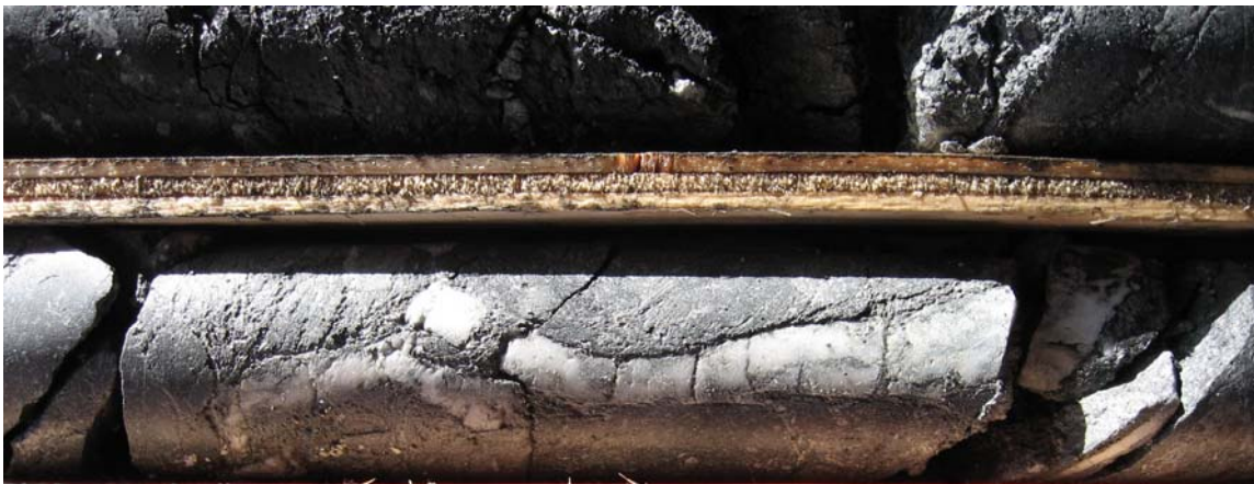
Figure 10 - 2007 Drill Core - Quartz vein cemented in gouge from SDN-07-04.
