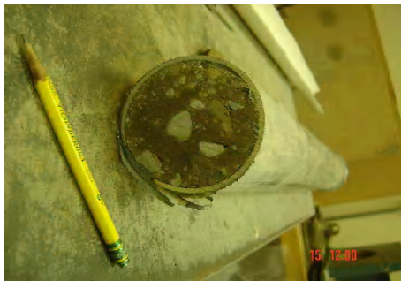
Extrude sample from tube
