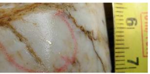
Figure 1: Visible gold in quartz; Sample 36528
