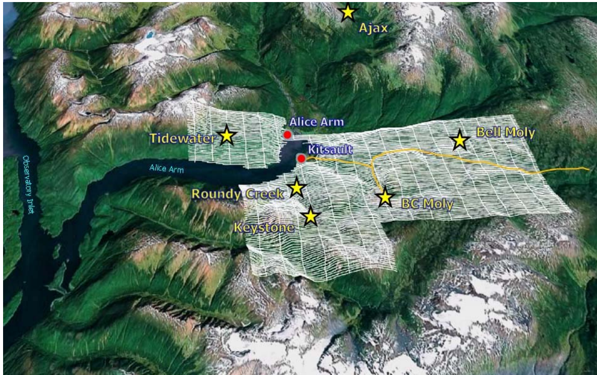
Figure 2: 2006 Aeroquest HELIMAG Survey Lines
