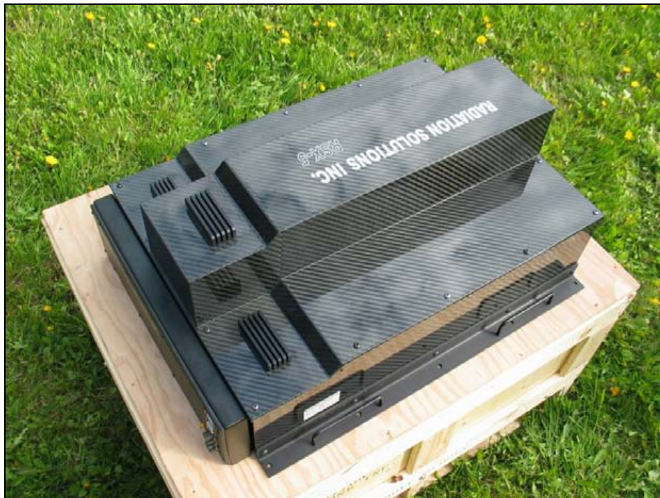
Figure 5 - Radiation Solutions RSX-5 Gamma Ray Spectrometer
