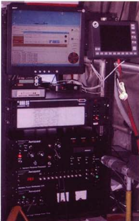
Figure 6. AeroTEM III Instrument Rack., including AeroDAS and RMS DGR-33 systems, AeroTEM power supply, data acquisition computer and AG-NAV2 navigation system.
