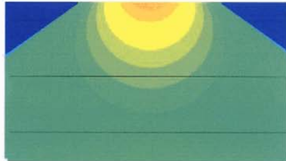
The footprint of a fixed-wing system is roughly 150 m on either side of the transmitter
