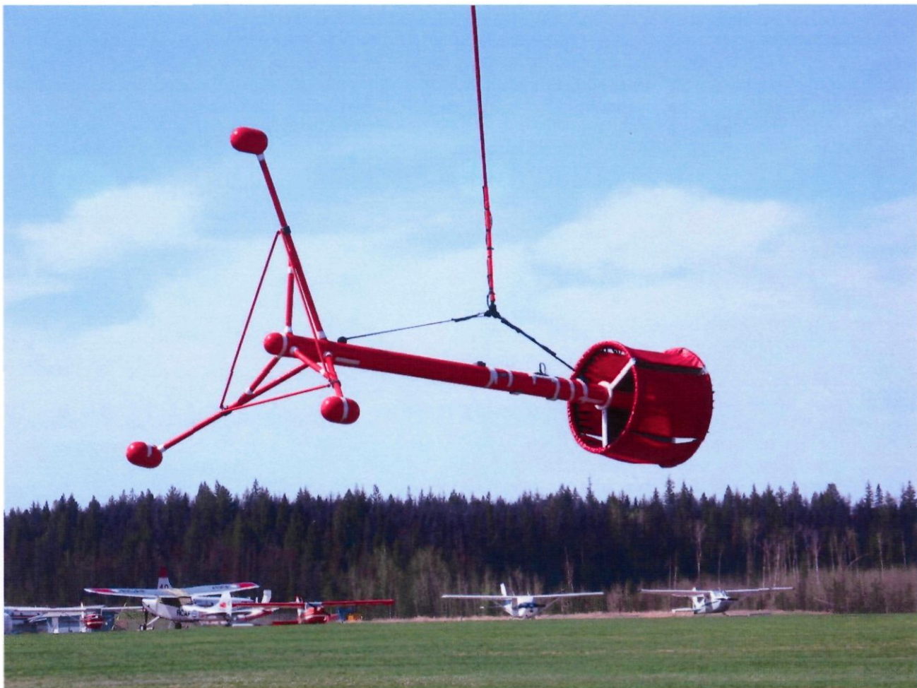
Figure 5 - The CMG tri-axial magnetic gradiometer.
