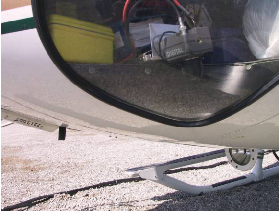
Figure 7. Digital video camera typical mounting location.
