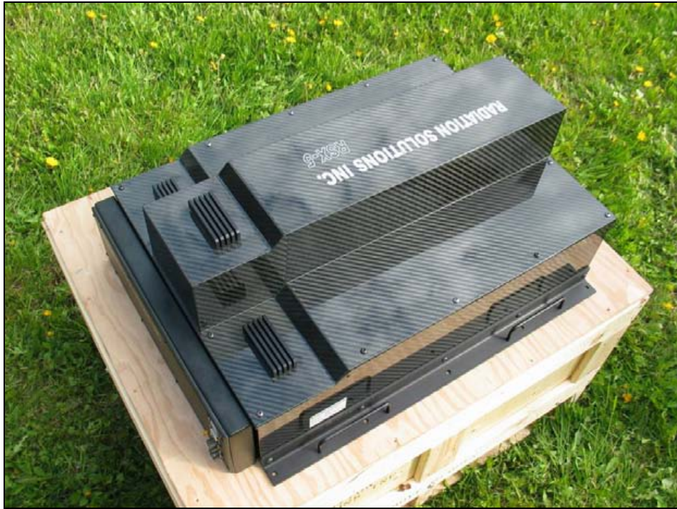
Figure 6 - Radiation Solutions RSX-5 Gamma Ray Spectrometer.
