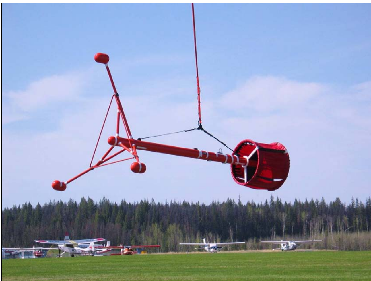
Figure 5 - The CMG tri-axial magnetic gradiometer.
