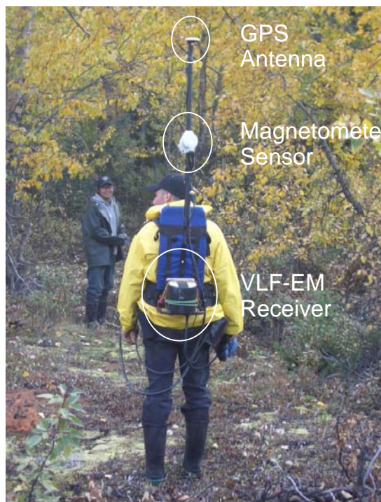
Figure 2: GSM-19 Overhauser Effect magnetometer and VLF-EM
