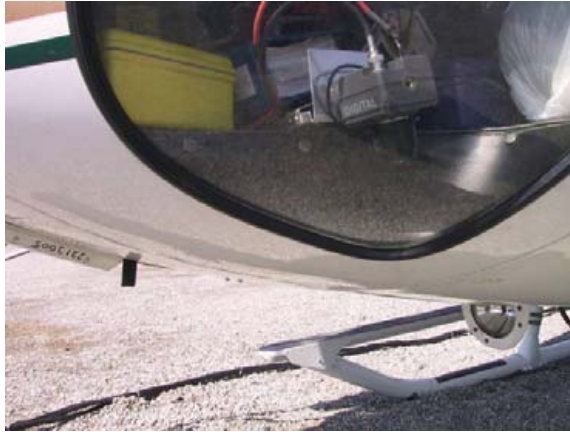
Figure 6. Digital video camera typical mounting location.
