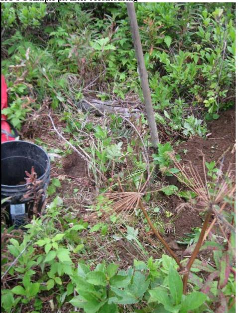
The volume was generally 5-10 litres in volume. The sample was classified by hand into the following screens: 2, 4, 8, 30 and 50. Some attempts were made to classify with 100 mesh, but it is very time consuming.
