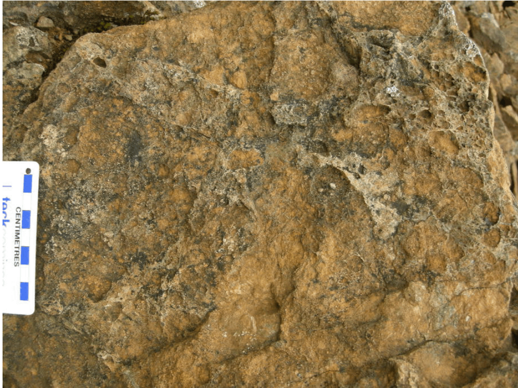
Figure 13. Intensely Fe carbonate altered and locally silica-flooded mafic fragmental rocks, near “Anomaly Creek,” along southwest margin of main Au-in-soil geochemical anomaly, Inlaw property.
