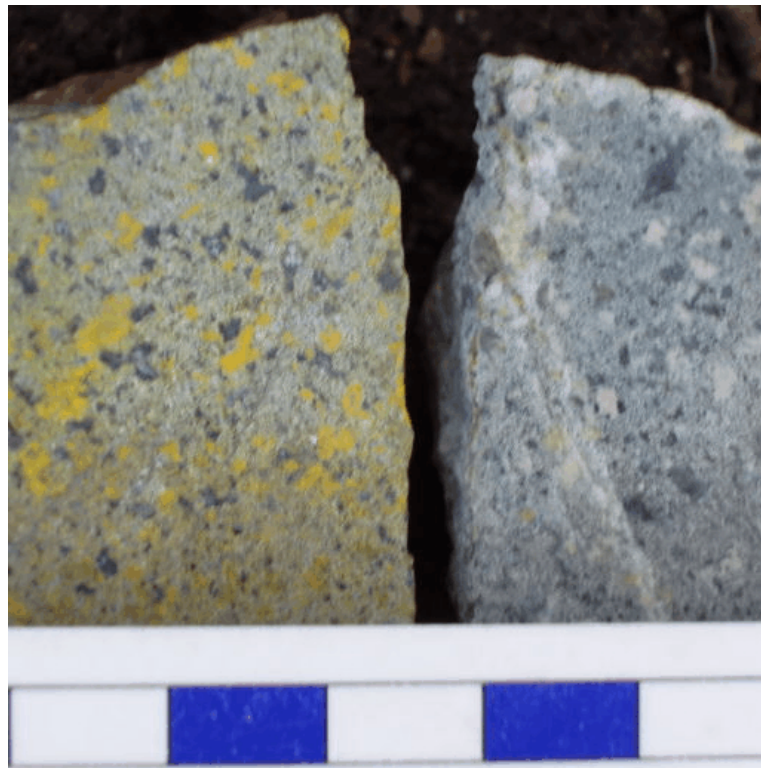
Figure 14. Stained (left) and etched (right) slabs of hornblende(?) - pyroxene feldspar bearing fine- to medium-grained monzonite or monzodiorite; bars at base are 1 cm.
