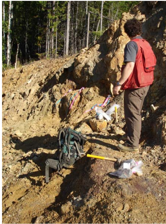
Plate 4: Sulphide Zone at the Borrow Showing looking east. Geologist is standing on the south contact and zone extends beyond outcrop face to east. Contiguous chips (flags in background) assay 1.50% Pb and 1.78% Zn across 3.0 metres.
