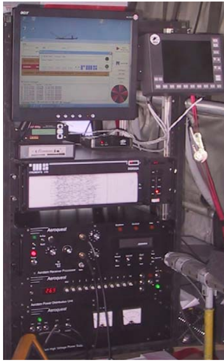
Figure 5. AeroTEM III Instrument Rack., including AeroDAS and RMS DGR-33 systems, AeroTEM power supply, data acquisition computer and AG-NAV2 navigation system.
