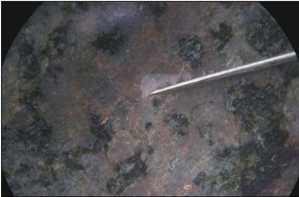
Photo 4 – Photomicrograph of finely disseminated metallic copper
