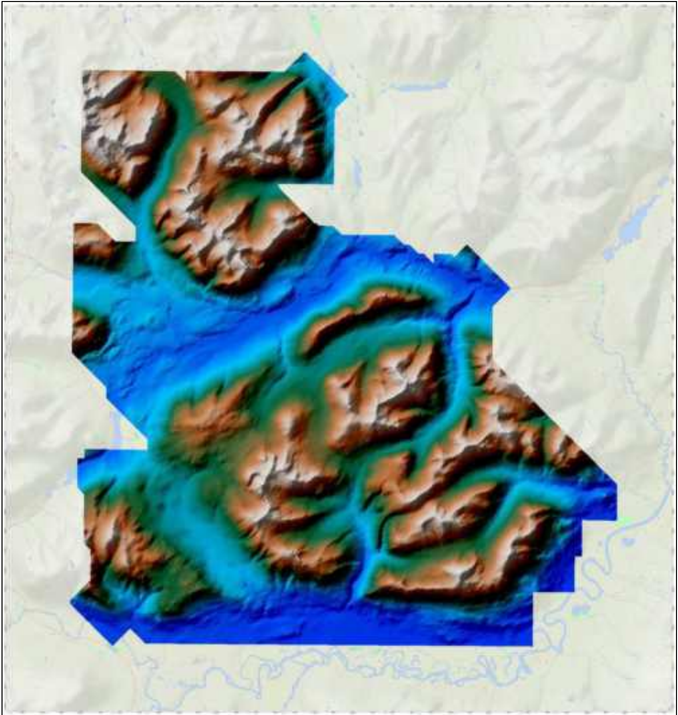
Figure 12 - Shaded image of the digital terrain model (DTM) over the Table Mountain survey area.
