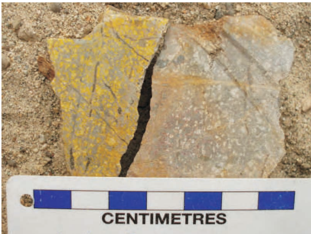
Figure 21. Slabbed and stained (left) sample of potassium feldspar porphyritic alkalic dyke, cut by quartz-pyrite-(chalcopyrite) veinlets, Krego zone, Dok property (59 ppb Au, 572 Cu).
