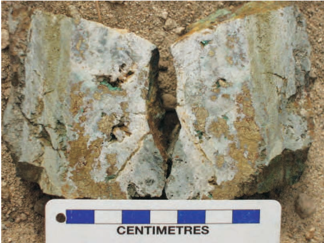
Figure 22. Slabbed and stained quartz calcite pyrite chalcopyrite vein cutting chlorite-epidote altered Stuhini Group volcanic rocks, south of Red Creek, southeastern Dok property; >40% Cu, 4.8 ppm Ag, only 13 ppb Au.
