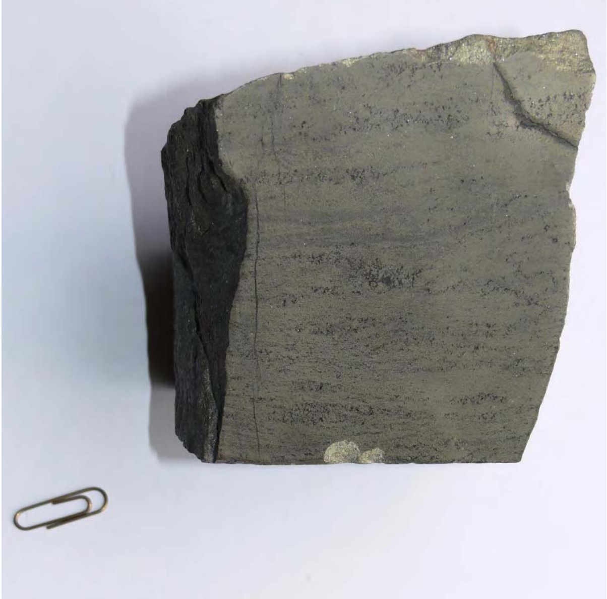
Figure No. 1 Banded massive sulphide from Frank Creek Discovery Trench. Sulphides in the rock consist mainly of pyrite, chalcopyrite and sphalerite.
