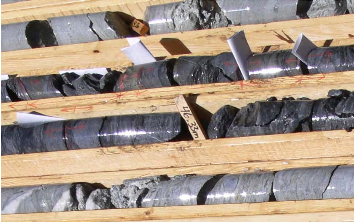
Figure No. 15 Sulphide Bands in Hole FC08-28, occurring in slump breccia at 44.8m, second column from top. The sulphides are mostly chalcopyrite. Lighter rocks above and below are silicified and sericitized.
