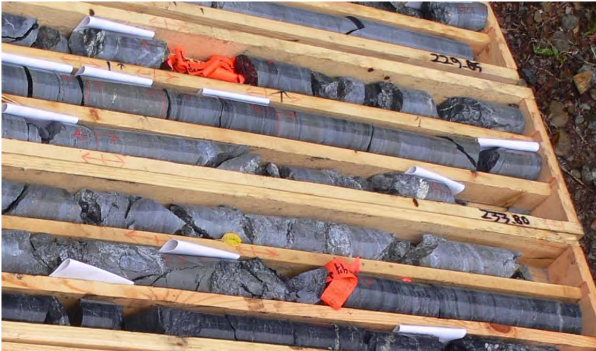
Figure No. 17 Sulphides in Hole FC08-29 occurring in apparently syngenetic bands near 232.3 m and associated with quartz veins at 236 m.
