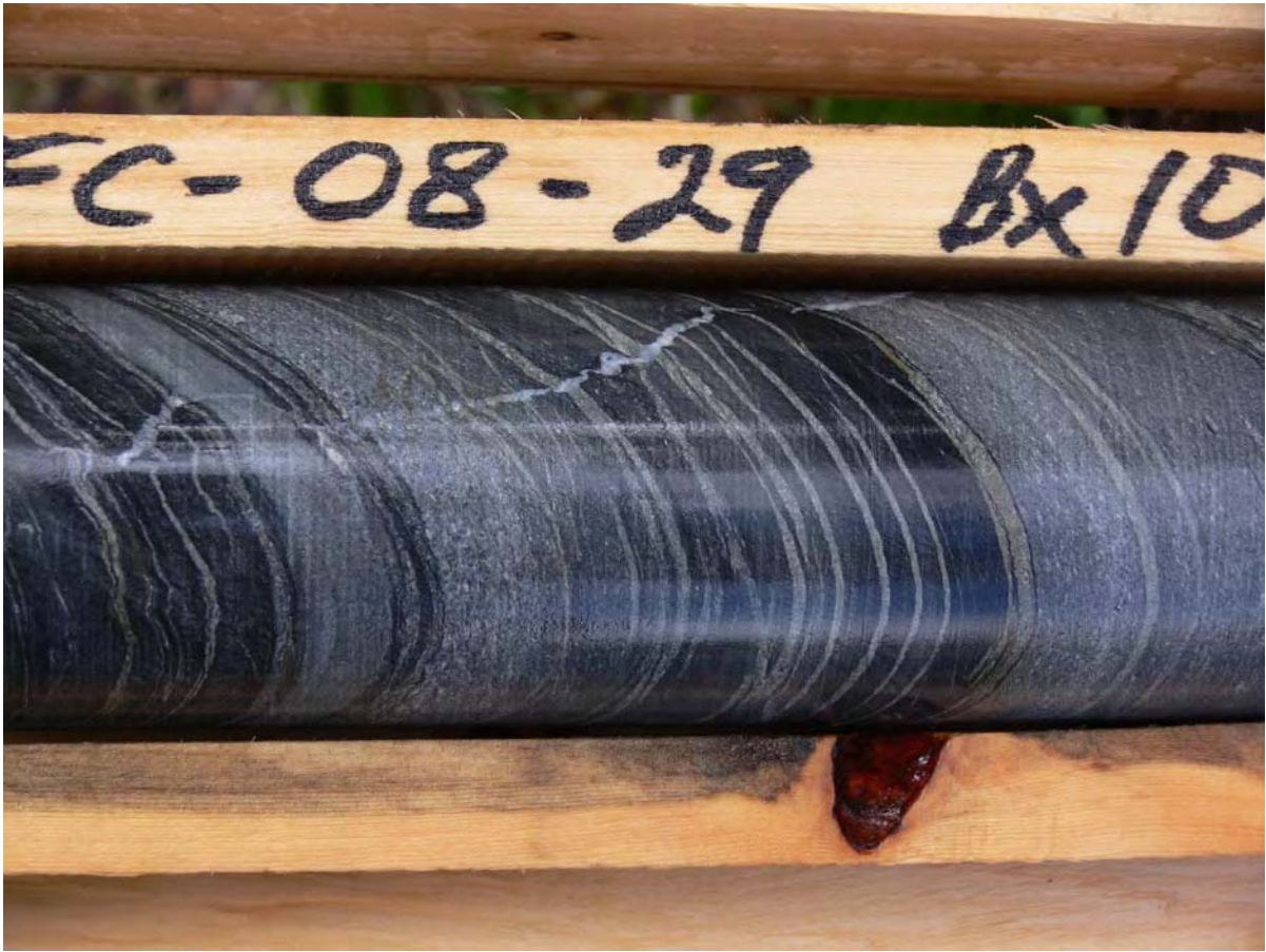
Figure No. 16 Graded Bedding in Hole FC08-29 with increasing fineness downward, evidence that rock strata are overturned.
