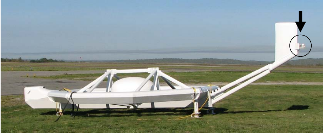
Figure 4. AeroTEM II EM bird. Arrow indicates the location of the second caesium magnetometer sensor.
