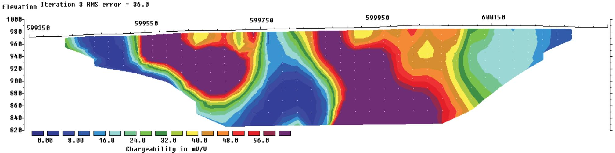
Unit Electrode Spacing = 25.0 m.
