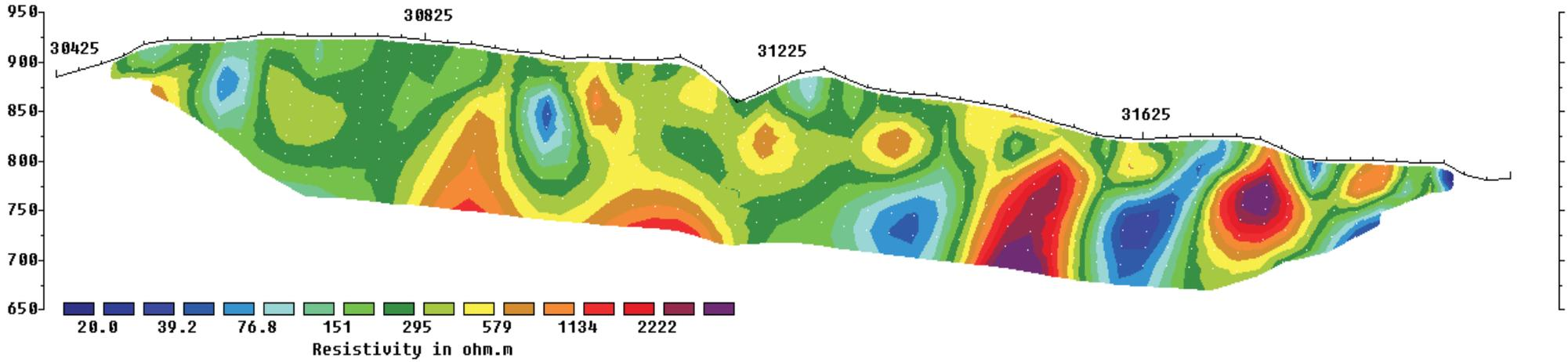
Unit Electrode Spacing = 25.0 m.
