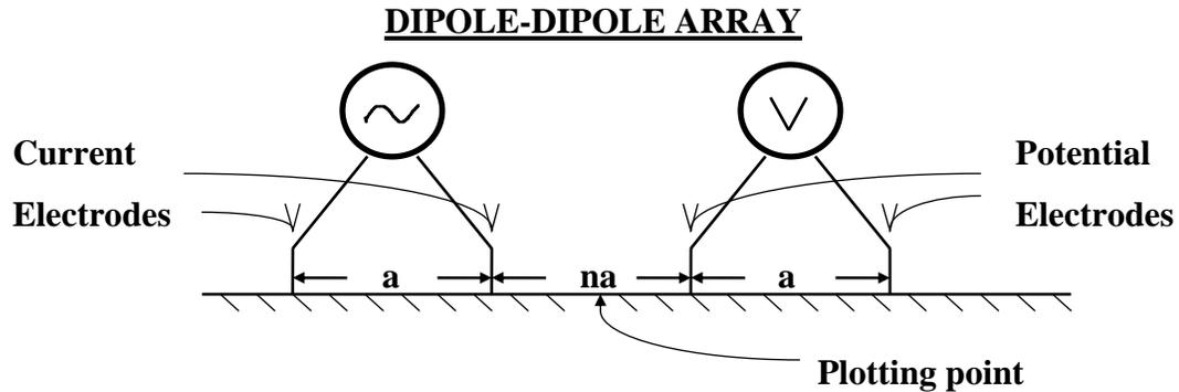
The electrode separation, or 'a' spacing, and reading interval were chosen to be 25 meters read to 12 separations (which is the 'na' in the above diagram). The theoretical depth penetration is about 115 meters, or 380 feet.
