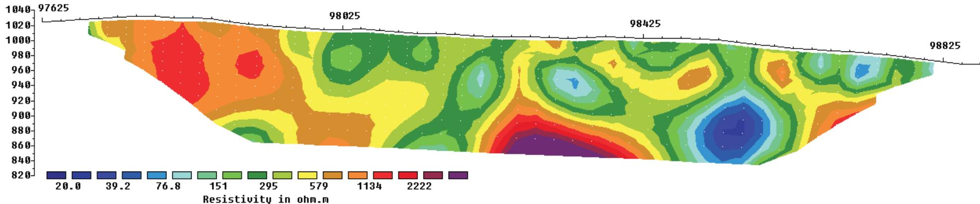
Unit Electrode Spacing = 25.0 m.
