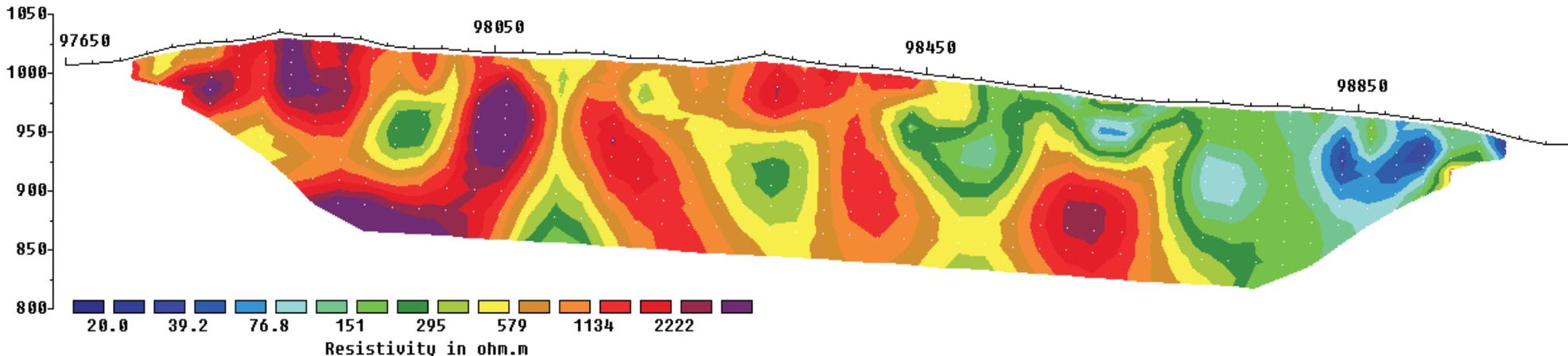
Unit Electrode Spacing = 25.0 m.
