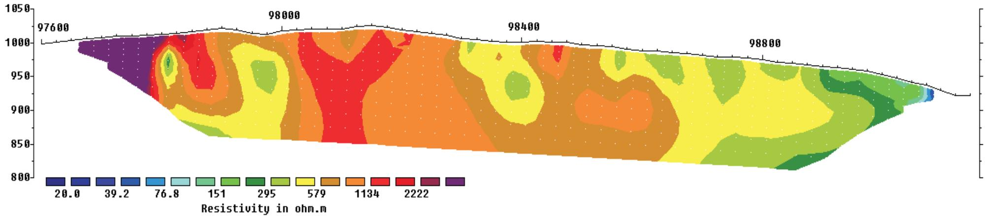
Unit Electrode Spacing = 25.0 m.
