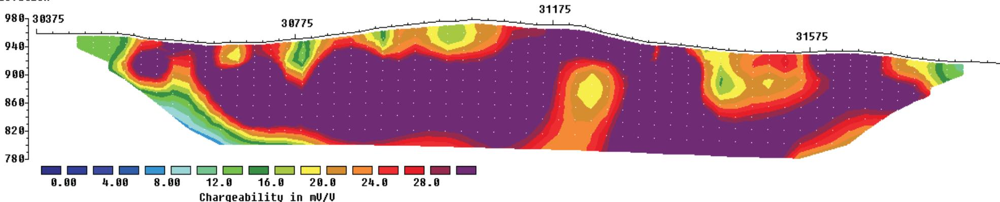
Unit Electrode Spacing = 25.0 m.
