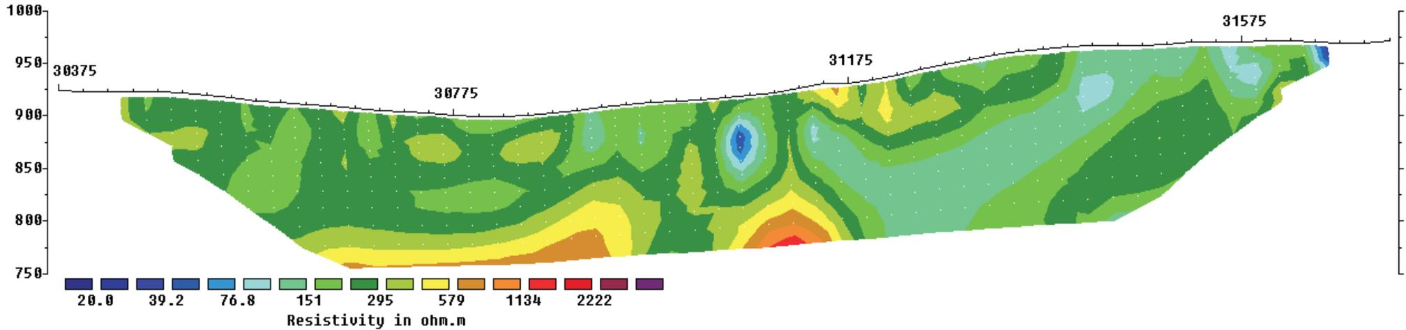
Unit Electrode Spacing = 25.0 m.
