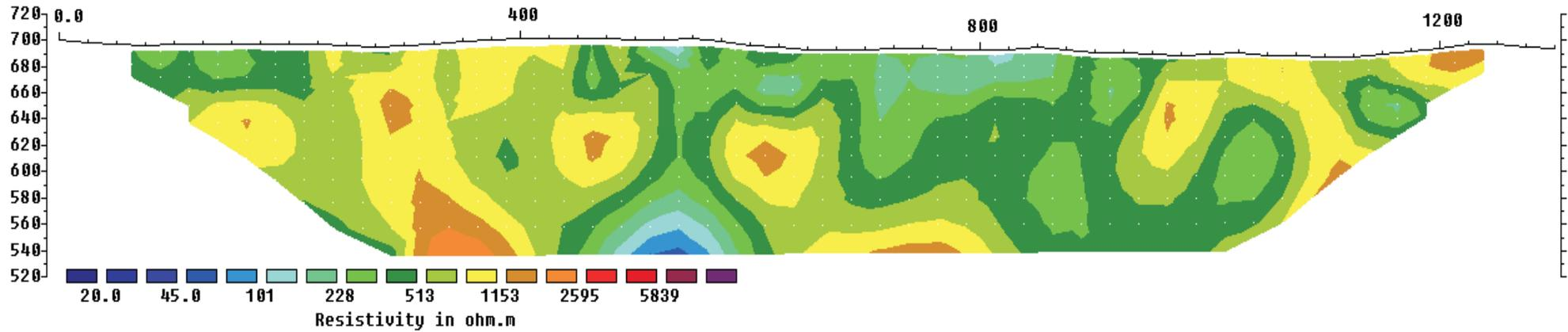
Unit Electrode Spacing = 25.0 m.
