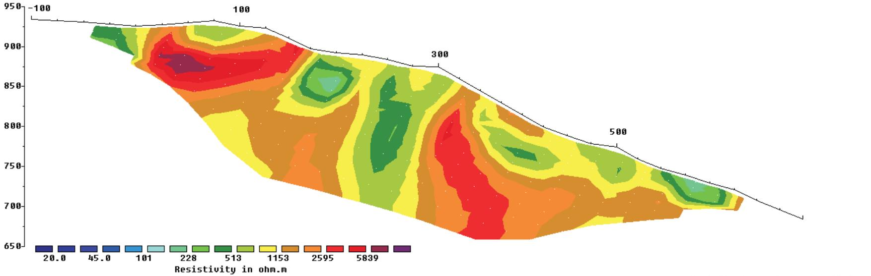
Unit Electrode Spacing = 25.0 m.
