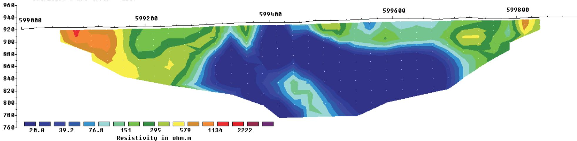
Unit Electrode Spacing = 25.0 m.
