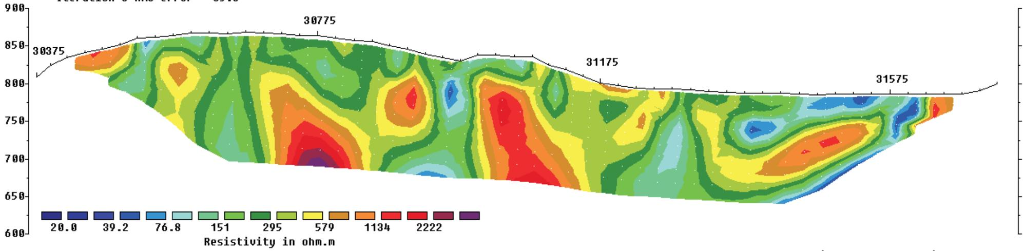
Unit Electrode Spacing = 25.0 m.
