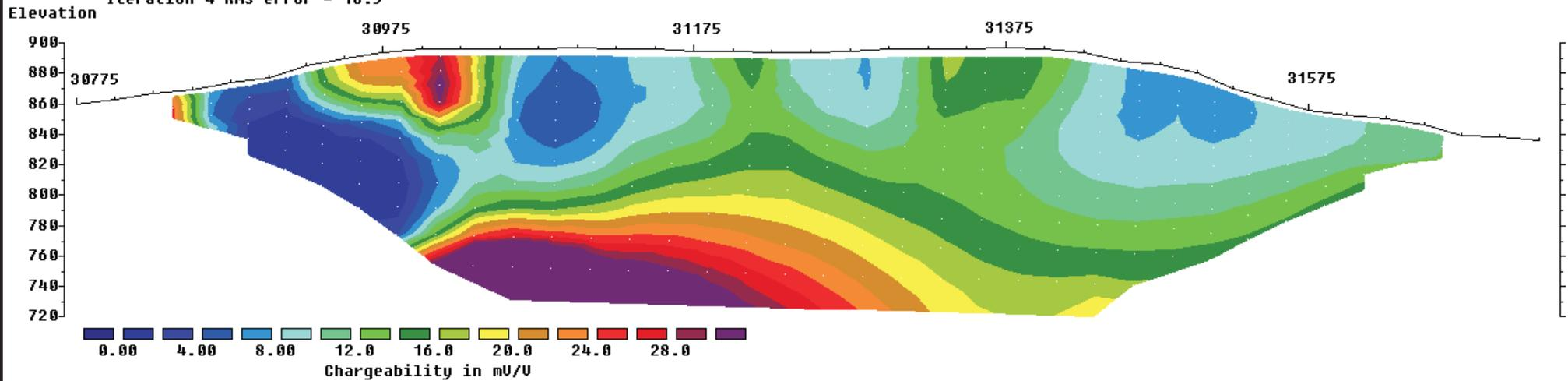
Unit Electrode Spacing = 25.0 m.
