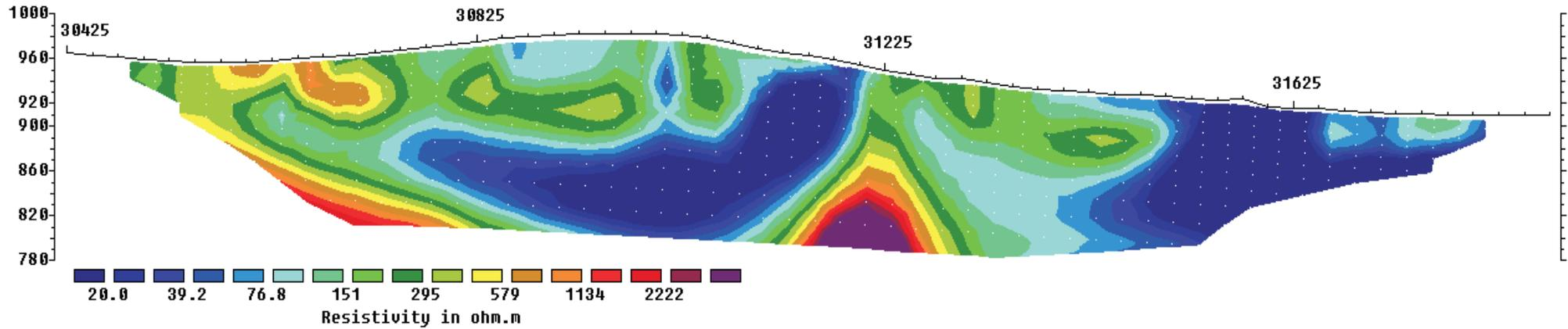
Unit Electrode Spacing = 25.0 m.
