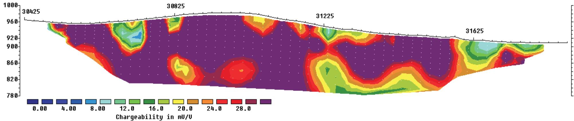
Unit Electrode Spacing = 25.0 m.
