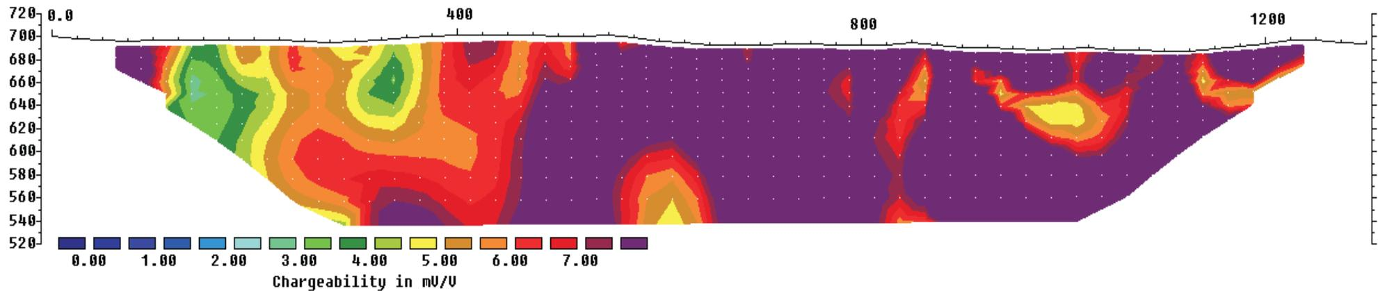
Unit Electrode Spacing = 25.0 m.
