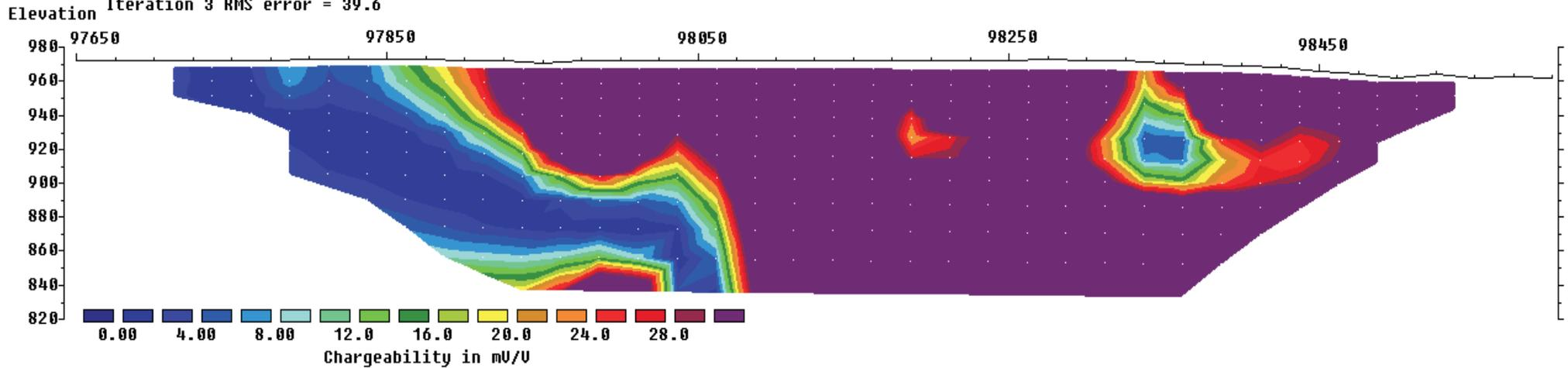
Unit Electrode Spacing = 25.0 m.
