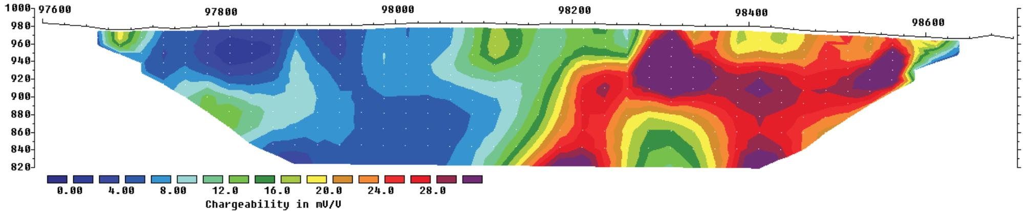
Unit Electrode Spacing = 25.0 m.
