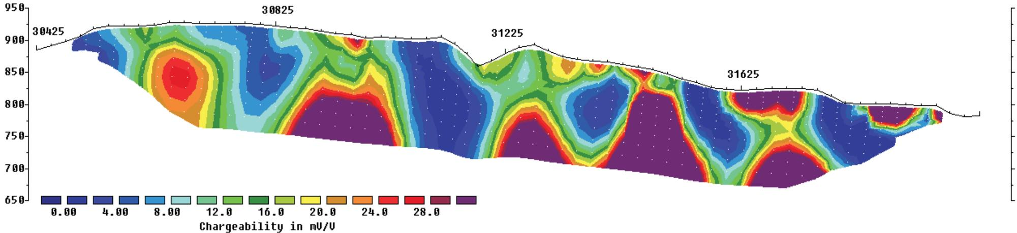
Unit Electrode Spacing = 25.0 m.
