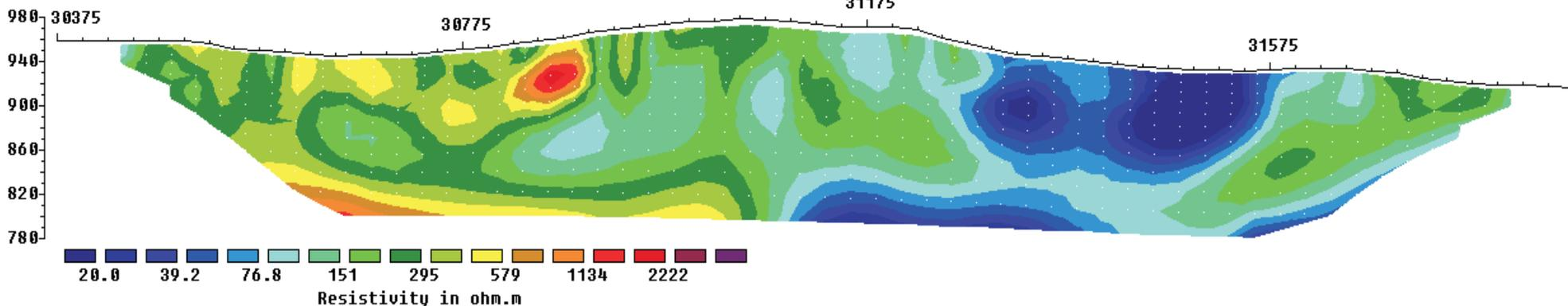
Unit Electrode Spacing = 25.0 m.
