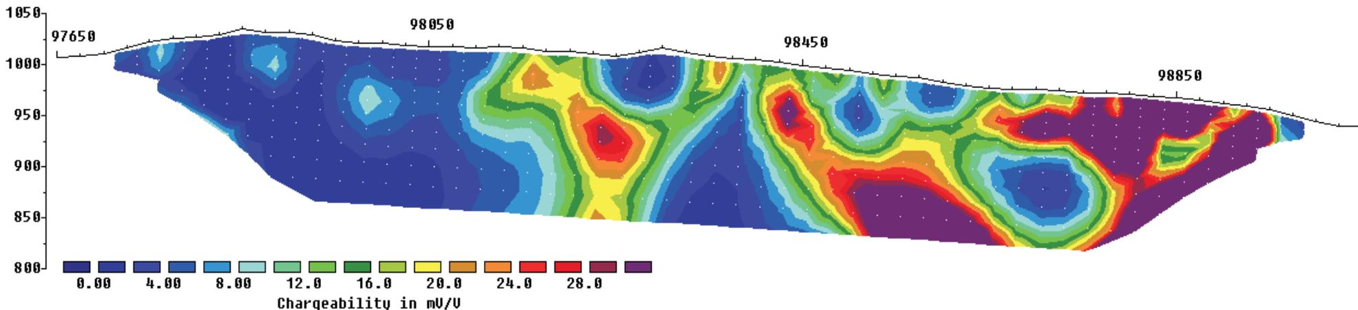
Unit Electrode Spacing = 25.0 m.
