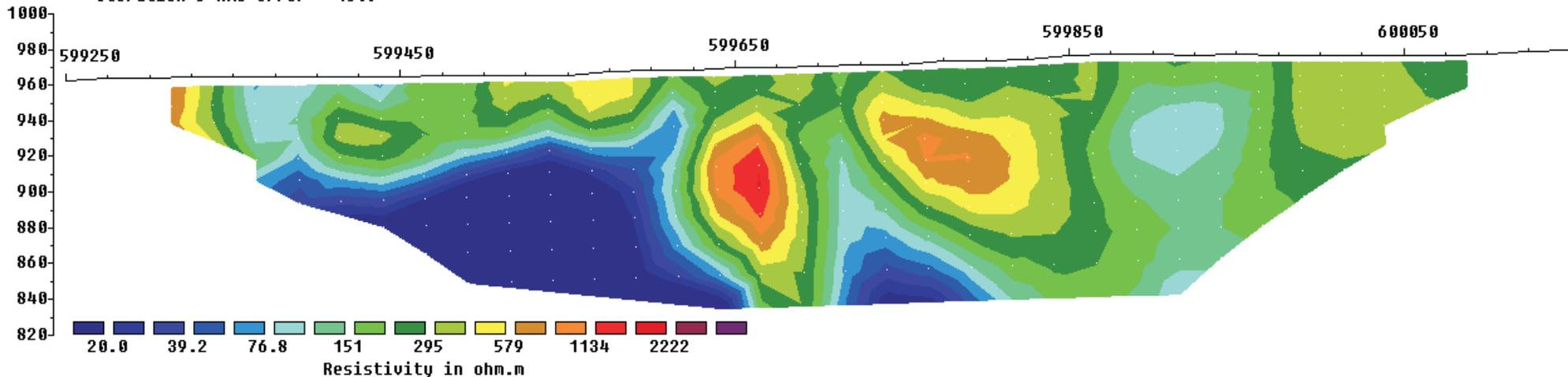
Unit Electrode Spacing = 25.0 m.
