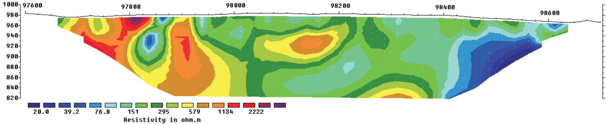
Unit Electrode Spacing = 25.0 m.
