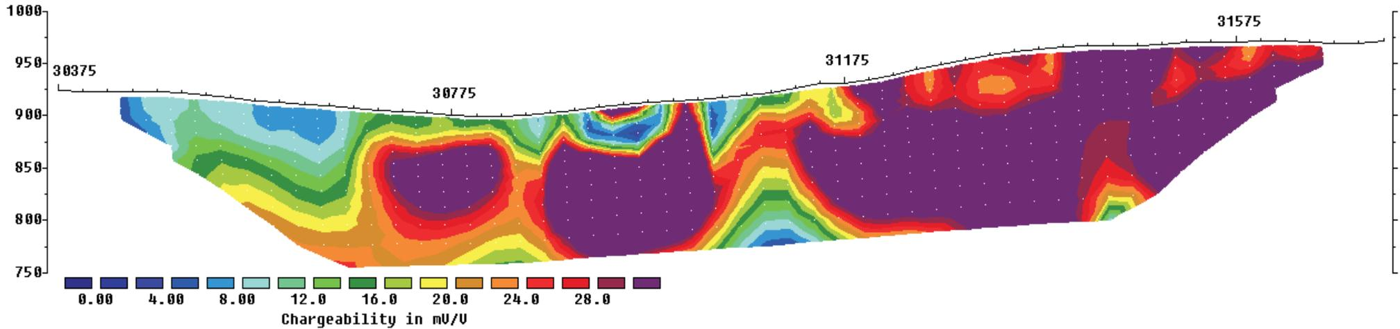
Unit Electrode Spacing = 25.0 m.
