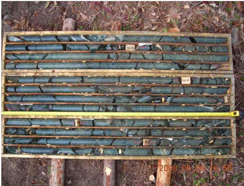
HAWK DDH 07-HK-02 Boxes 31 to 33 (154.84 m); EOH (NB boxes are lain out in reverse order, 33 at the top and 31 at the bottom)
