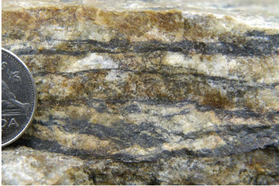
Figure 2: Tourmaline interlayered with quartz in quartz vein. This is evidence that the system was chemically open.
