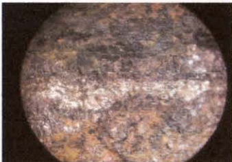
Microscopic photos of rock chip sampling – possible ultramafic
