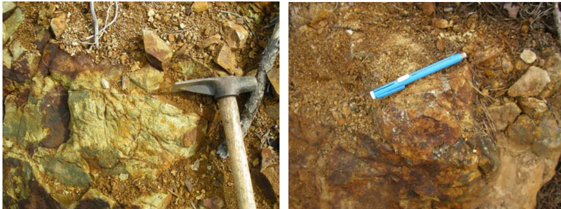
Figure 8. Photo: Mineralization at the Mustardo Showing. Left, porphyry with molybdenum bearing quartz stockwork veins, 346 ppm Mo (#43484). Right, sulphide stockwork veins in pyritized porphyry/andesite tuff, 0.95% Cu (#78290).
