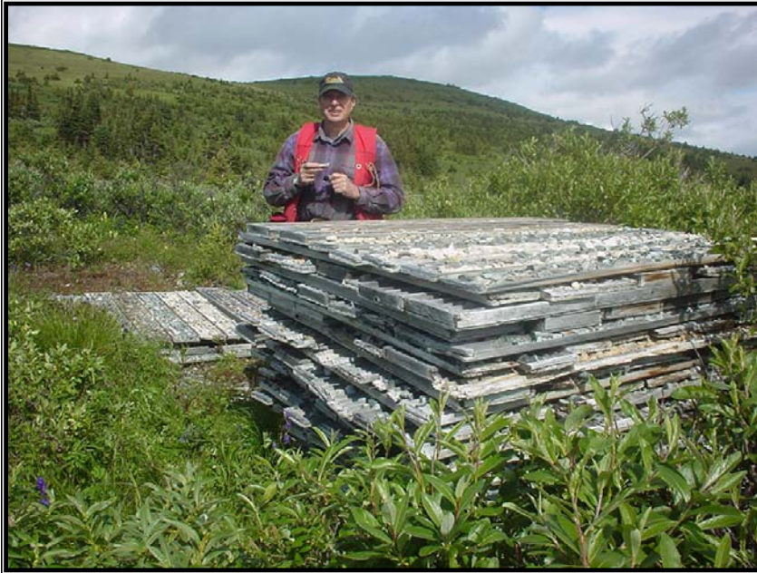
Figure 7. Brian Callaghan examines drill core stored on the property. The core, in boxes, is simply stacked in the open. In most cases box and footage labels are unreadable.
