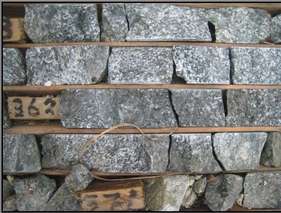
Figure 9. Hornblende diorite in Bing drill core. Note the foliation, melanocratic nature and actinolite veining. Footage labels are legible here, but not the box labels.
