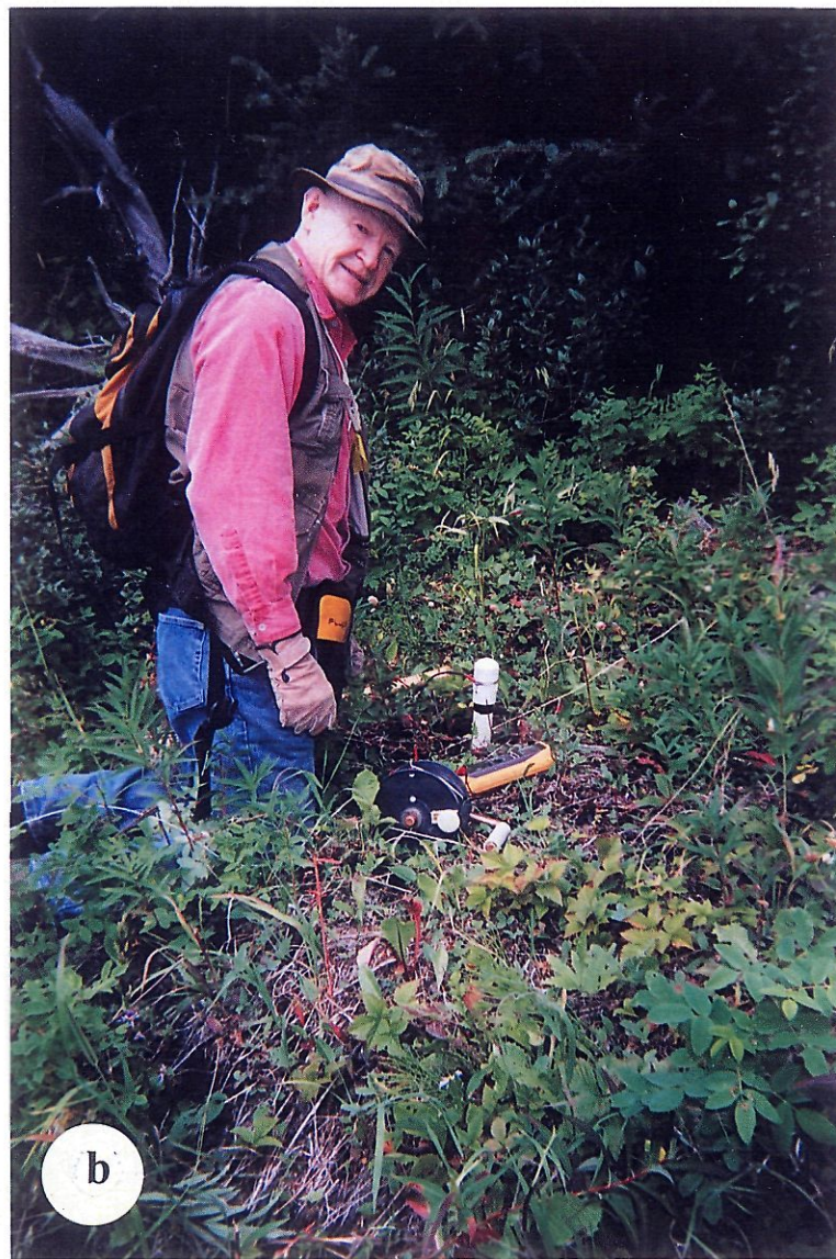
Photos 2a,b Self Potential Operation (a) reel, (b) voltmeter and electrodes
