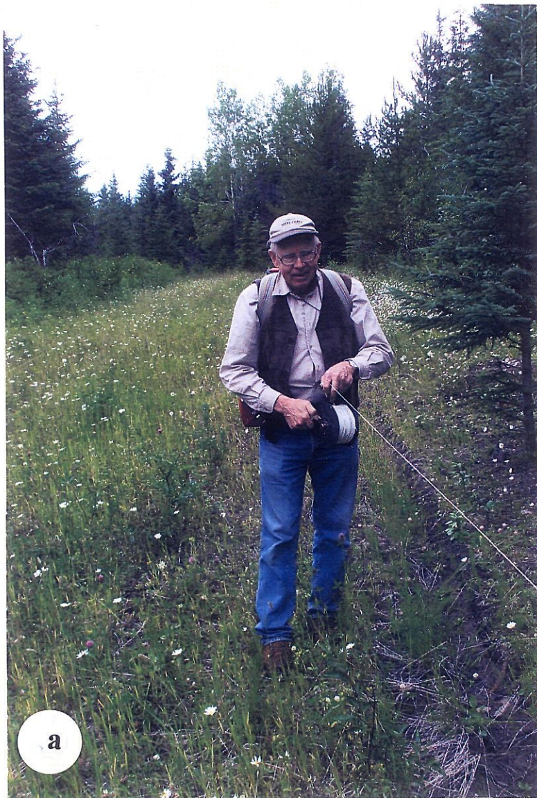
Photos 2a,b Self Potential Operation (a) reel, (b) voltmeter and electrodes
