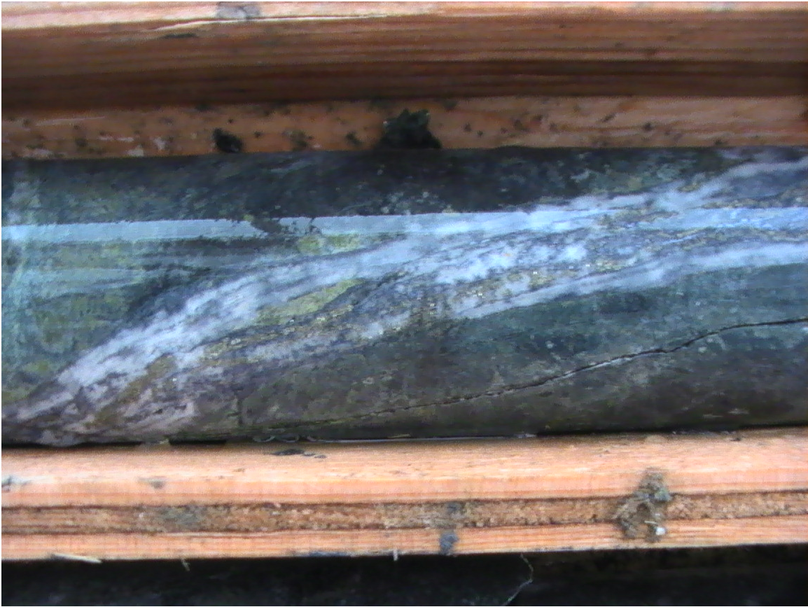
Photo 5: Molybdenite and pyrite in quartz vein
