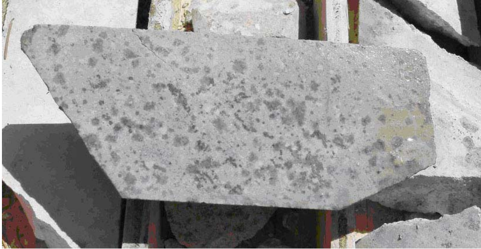
Plate 3. Fine-grained quartz porphyritic dyke. Blue-green aggregates are a clay-sericite assemblage, and small dark flecks are iron-copper-gold sulphides/sulphosalts. This alteration style is common in higher grade mineralized zones.
