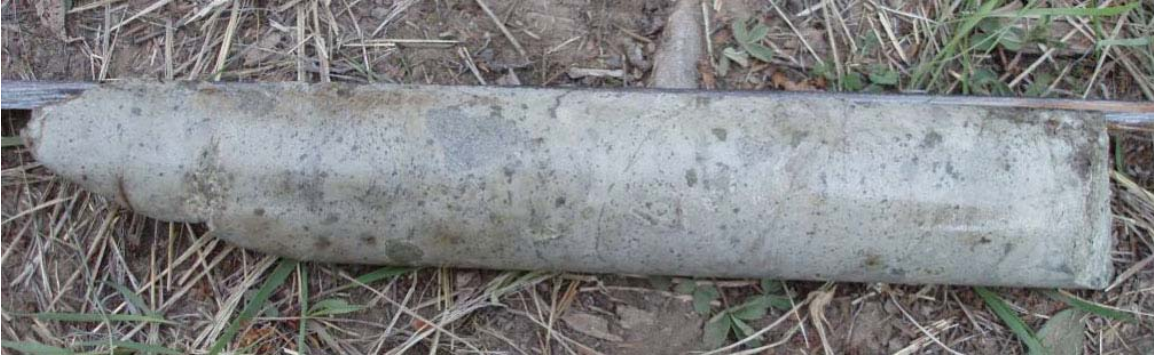
Plate 1. Clay-silica altered subaerial volcanoclastics. This unit may be one of the principle hosts to strong mineralization in holes 06-12 and 06-03.
