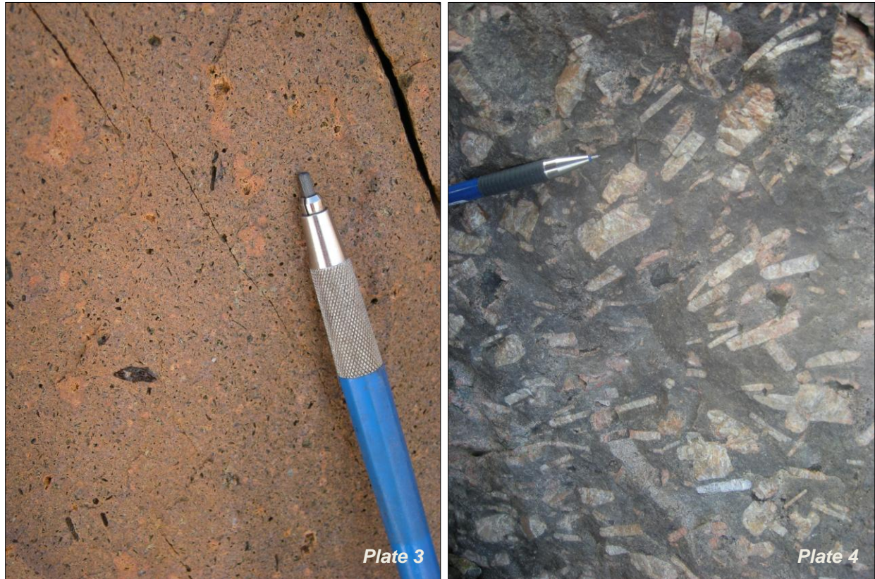
Plate 3: Late biotite-phyric syenite dyke crosscuts intrusive breccia
