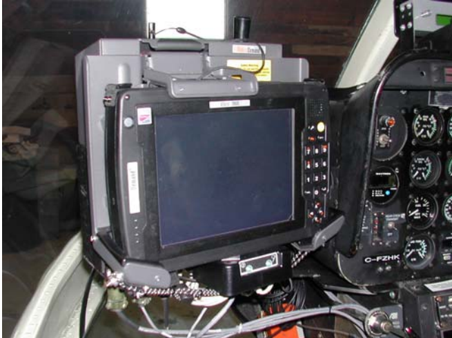
Figure 4: AGIS installed in the Bell 206.
