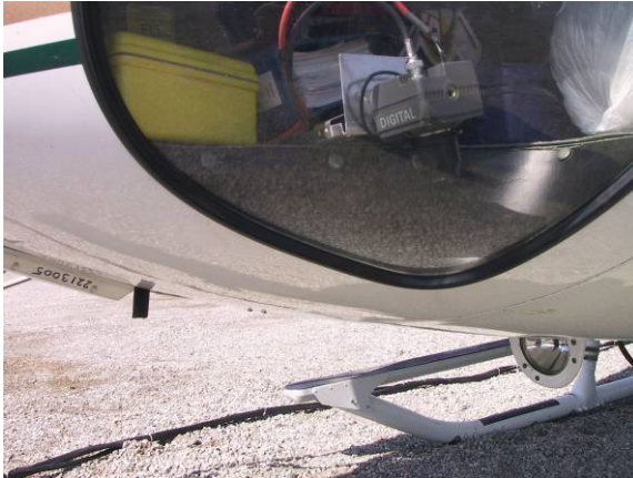
Figure 6. Digital video camera typical mounting location.
