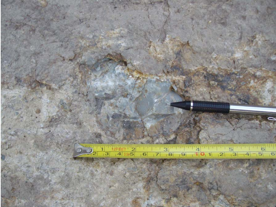
Figure 8 : Photo of 8 cm siliceous fragment from the west end of trench L609-XT-10 which may in part be responsible for 1.54 g/t Au over 1.5m.
