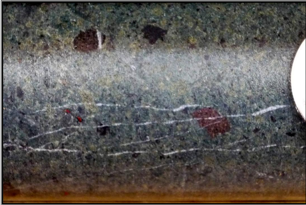
Figure 28. Crystal lithic tuff from RVC 08-18 about 15 m depth.
