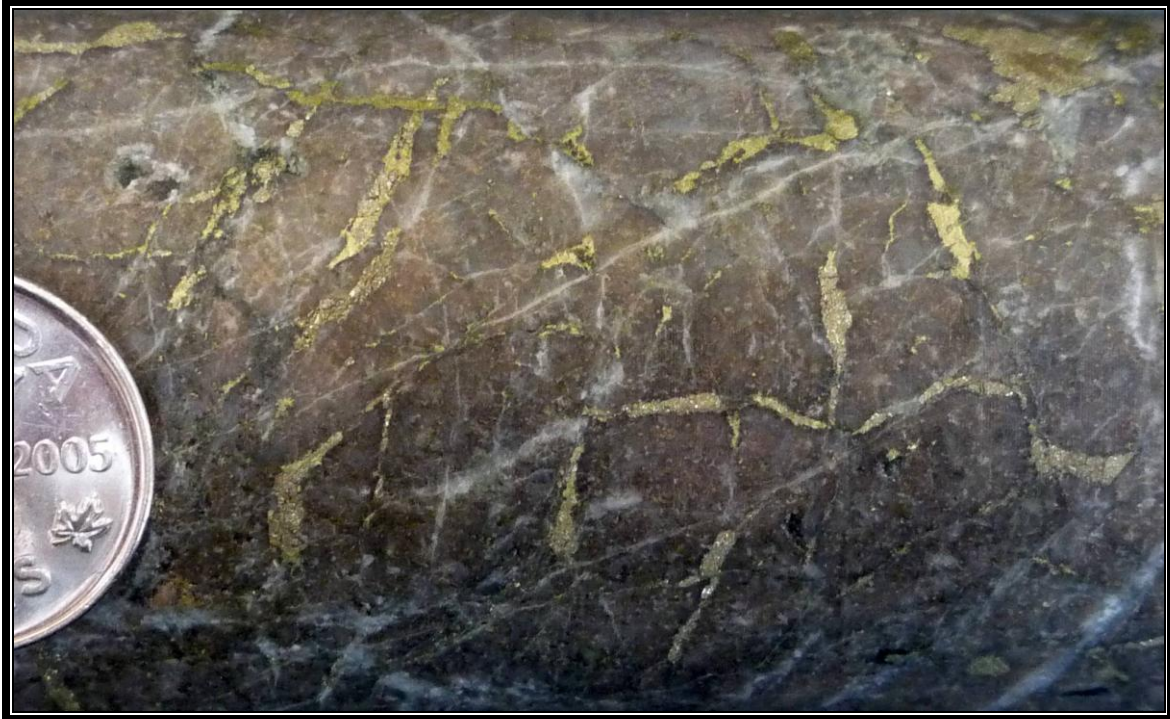
Figure 39. Chalcopyrite (brighter yellow) and pyrite (lighter yellow) as fracture fillings in monzonite. RVC 08-10 @ 405m.
