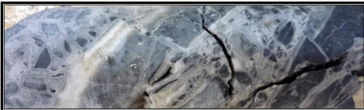
Figure 36. Chalcedonic quartz in a fault from RVC 08-19 @ 382 m. This alteration is fracture and fault controlled and has local open space. It was formed late.
