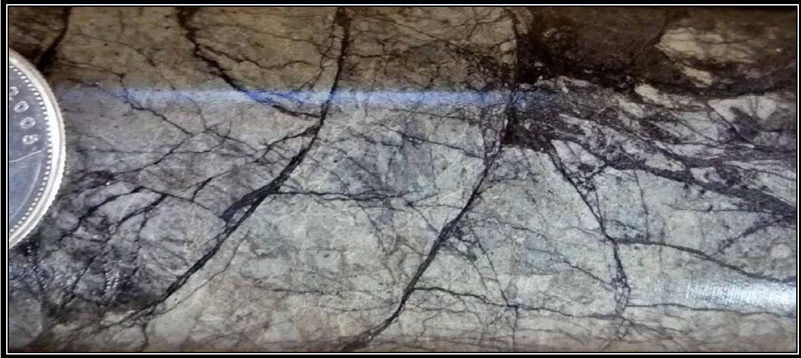
Figure 19. Monzonite jigsaw fit breccia at about 60 m in RVC 08-16.
