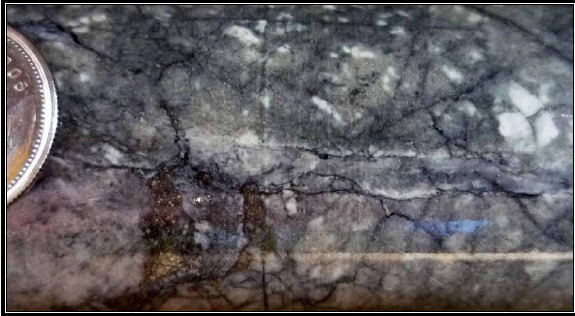
Figure 21. Jigsaw fit monzonite breccia with anhedral white plagioclase phenocrysts and fracture fill pyrite.
