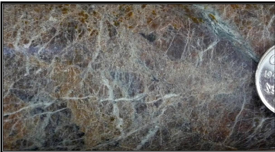
Figure 35. RVC 08-19 @ 240 m showing potassic and chlorite alteration of monzonite. This is an example of the productive part of the hole showing intense alteration and rebrecciation with quartz flooding.
