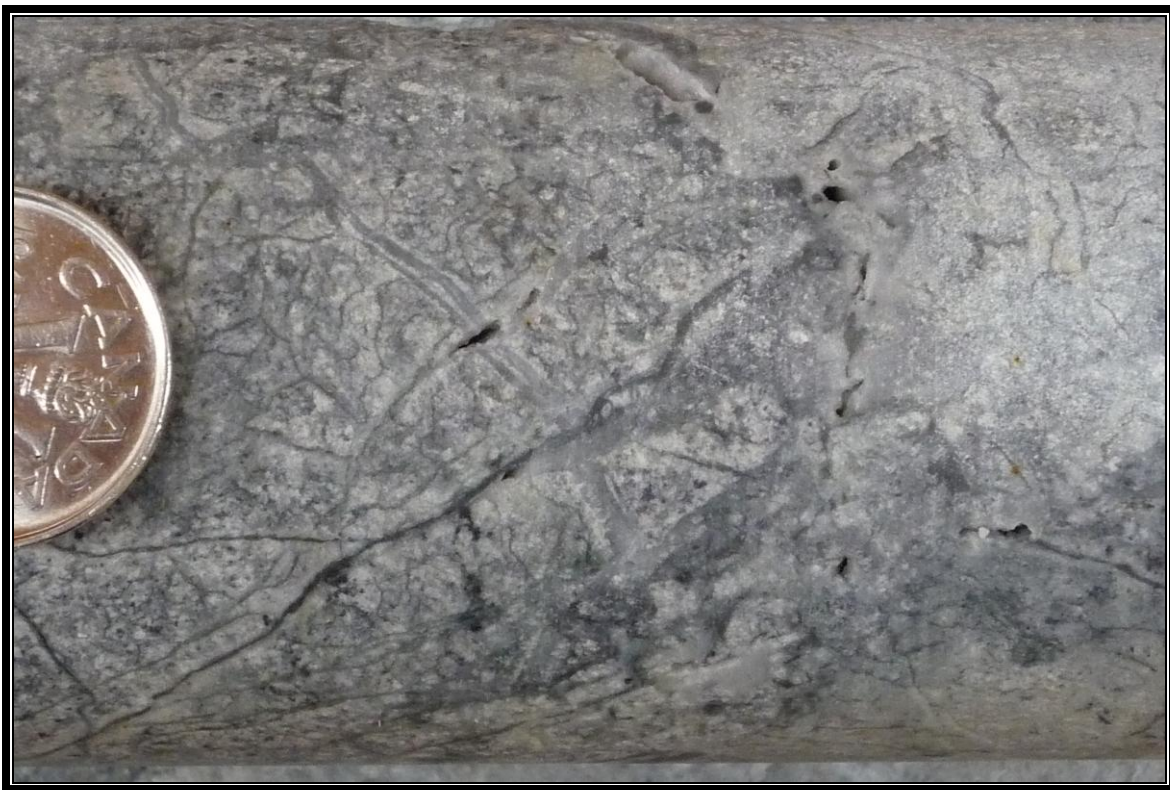
Figure 40. RVC 08-19 @ 360 m shows silica flooding in monzonite.
