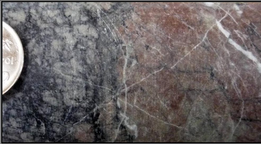
Figure 33. RVC 08-19 @ 37 m showing potassic alteration of monzonite with quartz flooding in narrow irregular veinlets.
