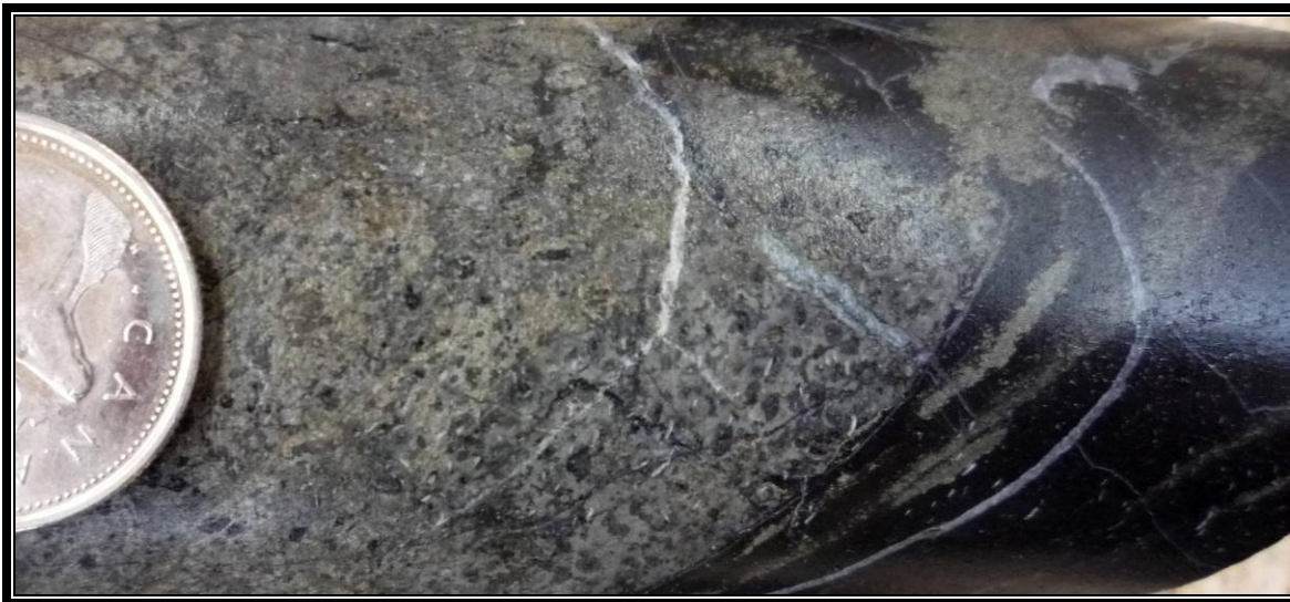
Figure 23. Contact between diorite (left) and pyritic argillite (right- black) at 158 m in RVC08- 16. Note the absence of baking of the argillite, and the lack of deformation, brittle or otherwise at the contact. Also note the fine grained pyrite bands parallel to the contact along bedding in the argillite.
