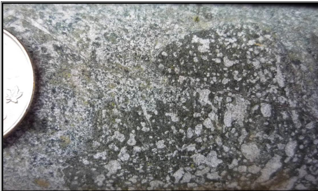
Figure 29. Augite basalt from RVC 08-18 about 45 m depth showing calcite vesicle and cavity filling in breccia.
