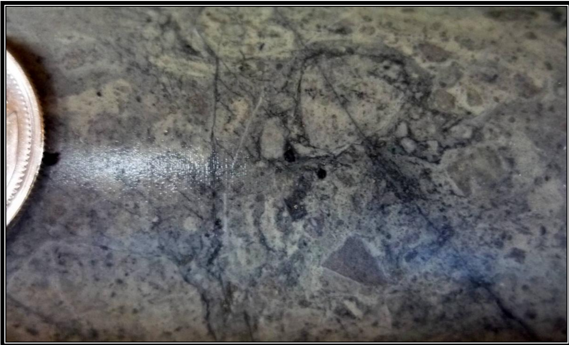
Figure 20. Monzonite breccia at about 85 m in RVC 08-16 showing disaggregated monzonite clasts in monzonite matrix.
