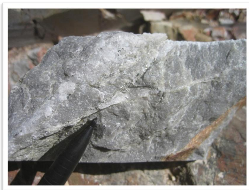
Figure 6. Silicification with disseminated pyrite on a fresh surface of sample 09HLB5 (1.74 g/t Au) from the Heart Lake zone.
