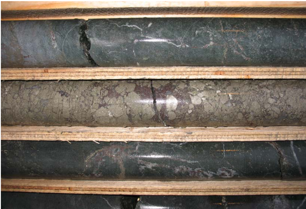
Plate 3: Photo shows well mineralized zone at 237 m in drill hole SK09-01. Semi-massive to massive sulphide mineralization consists of pyrite-sphalerite-chalcopyrite-minor galena with traces of visible gold in some zones. As well, quartz-calcite stringers with sphalerite and pyrite can be seen in the surrounding core interval. Core is NQ size.
