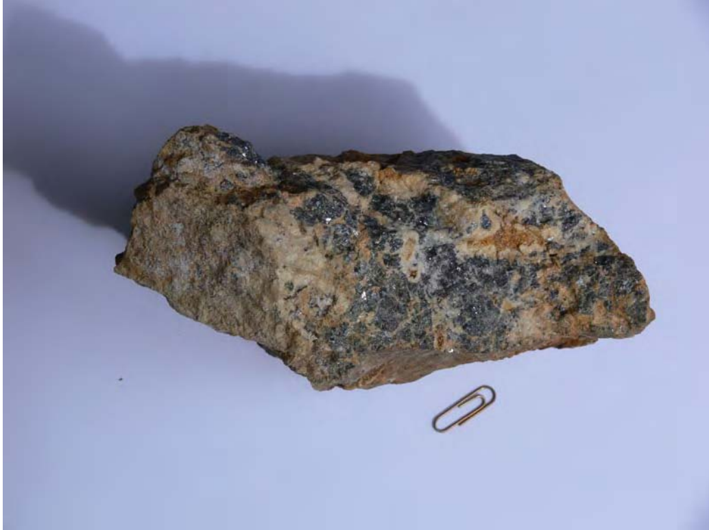
Plate No. 1 Cariboo Property. Sphalerite and galena in carbonate vein breccia, from Main Showing outcrop.
