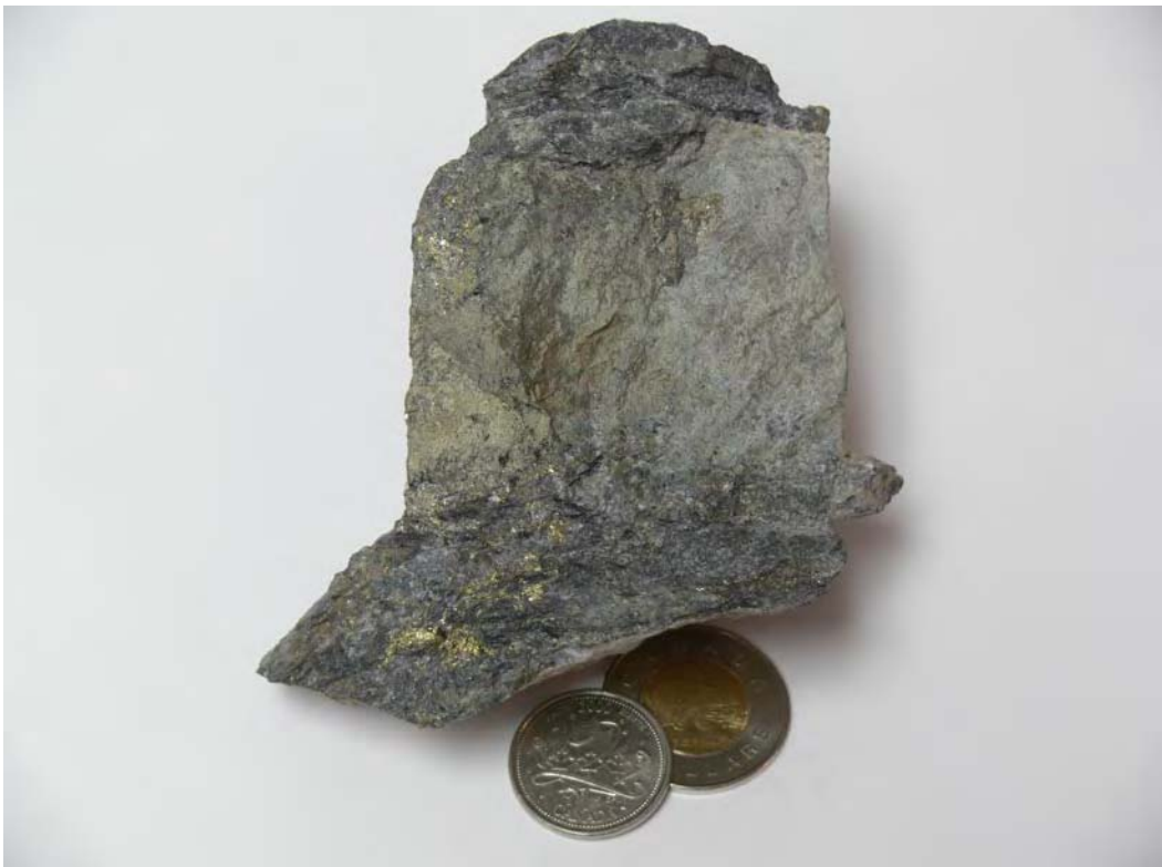
Plate No. 2. Fine grained massive chalcopyrite and pyrite layer in quartz muscovite schist from the Discovery Trench. Coarser vein chalcopyrite in the lower part of the specimen appears to be later. The massive sulphide layer is gently warped along with the rock's foliation.
