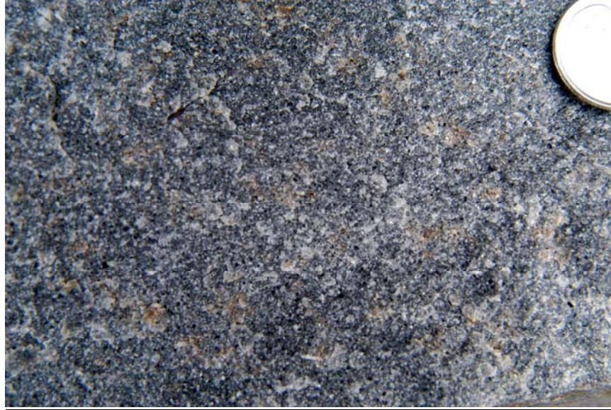
Figure 17: Kootenay King quartz-arenite illustrating medium-grained, homogeneous character with approximately 10-15 percent black, lithic grains. See figure 5 for location.
