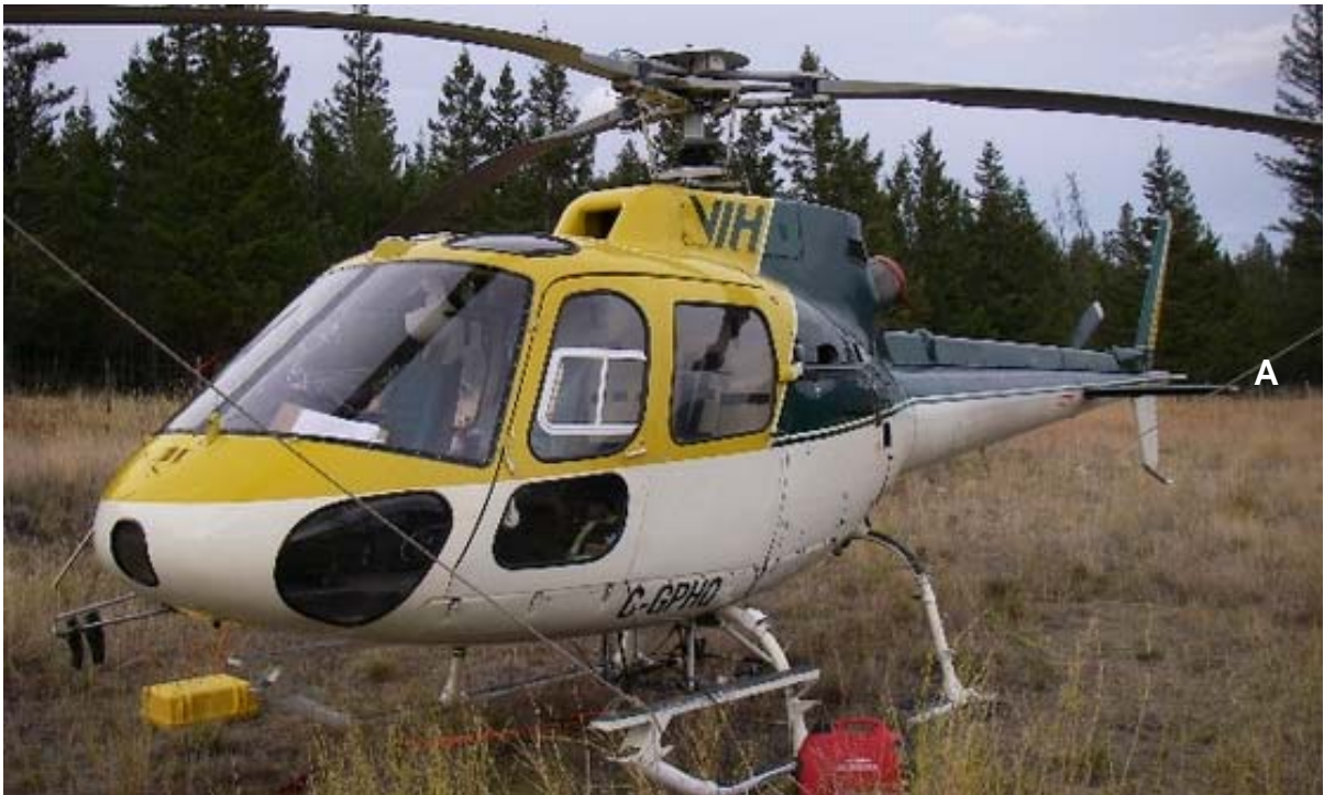
Figure 2. Survey aircraft C-GPHQ showing magnetometer stinger (A)
