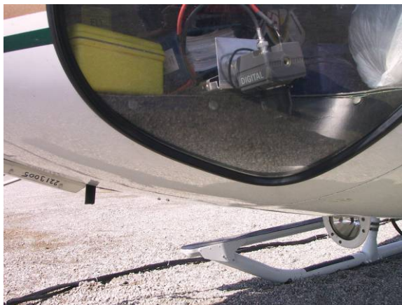
Figure 7. Digital video camera typical mounting location.
