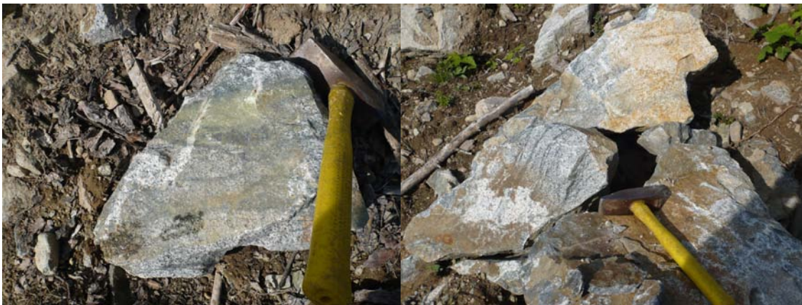
Station 5: (left) Banded (skarn-like) green epidote + trace disseminated chalcopyrite in monzodiorite. (right) Wavy massive veinlets of magnetite in monzodiorite + epidote + trace chalcopyrite
