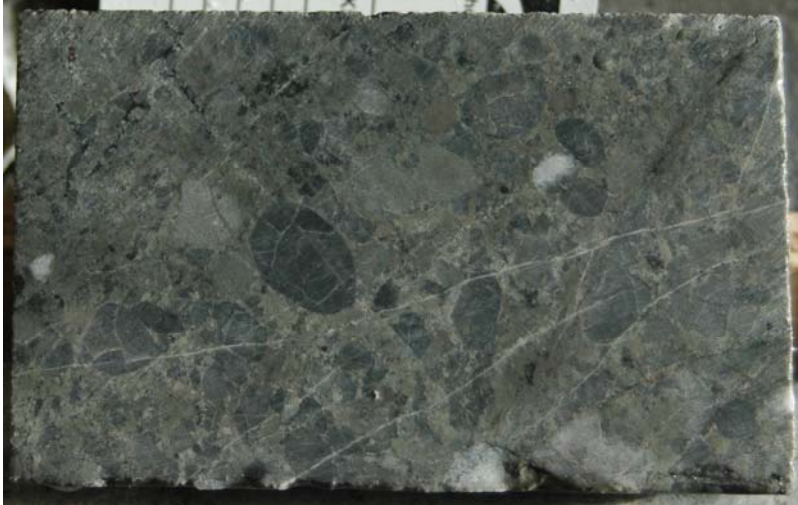
Plate 1. Polymictic epiclastic from hole 9013, 245.5-245.6 m. Sample is at true scale.
