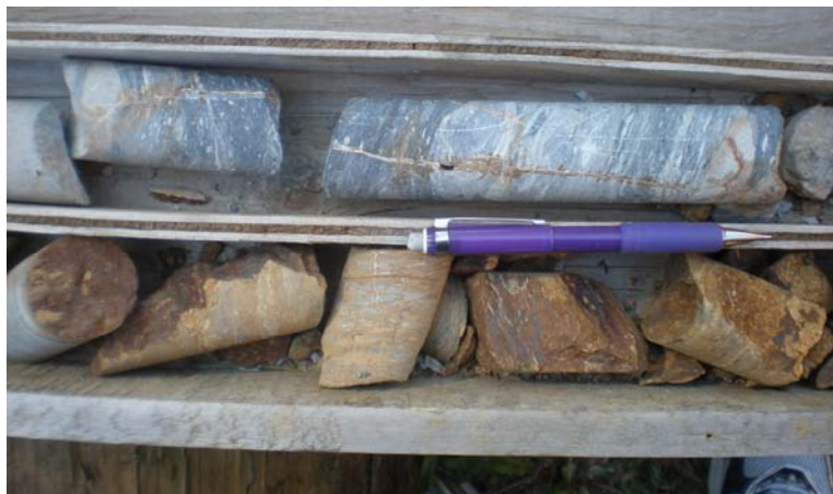
Plate 1. Drill core of strongly foliated and tectonized graphitic mudstone and siltstone from drill hole CZ-10-2, CZ property. Note orange to brown Fe oxide on fracture faces and foliation planes in core below mechanical pencil.
